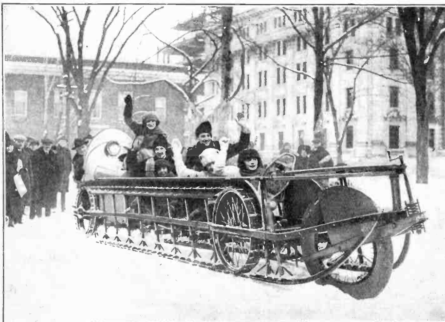
Equipped with caterpillar treads and a husky motor, the sled shown in the above illustration is capable of carrying its passengers over hill and dale at the rate of twenty-five to forty-five miles an hour. The large wheel at the front rests on springs and is used to steer the sled. It was shown at the Winter Carnival at Montreal, Can.
