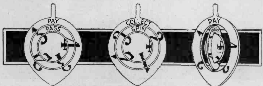
The three concentric disks fastened to a common shaft and arranged with numbers is the latest in gambling devices. The illustration above shows how it designates the "put and take."
