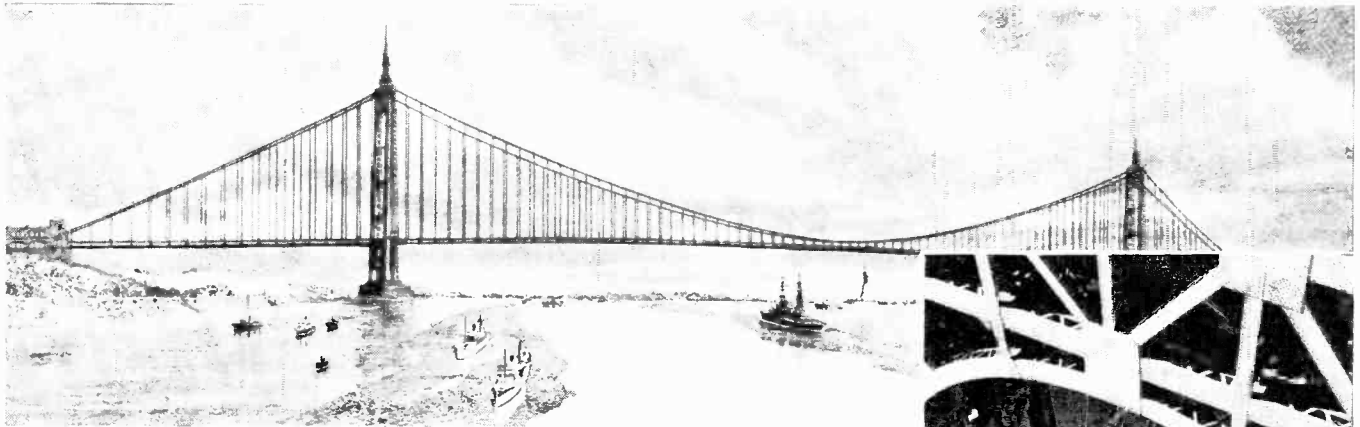
$60,000,000 will be the cost of the proposed Liberty Bridge, which will span the Narrows and link Brooklyn with Staten Island. The towers will be 800 feet high—taller than the Woolworth Building—and the main span 4,500 feet long—1,000 feet longer than that of the Hudson Bridge. Original features will be a carillon of bells and a beacon light. (Robinson and Steinman, Engineers.)
