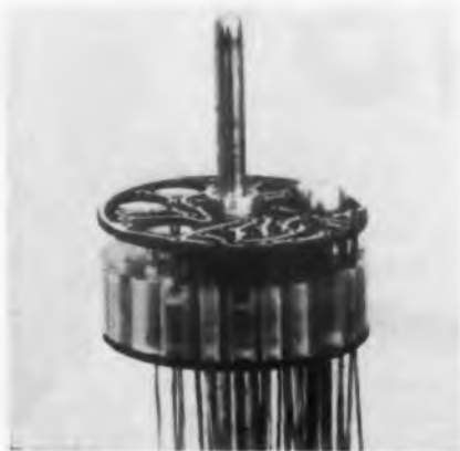
Fig. 7. The top printed-wire plate has been added and pin No. 2 has been threaded into pin No. 1.
