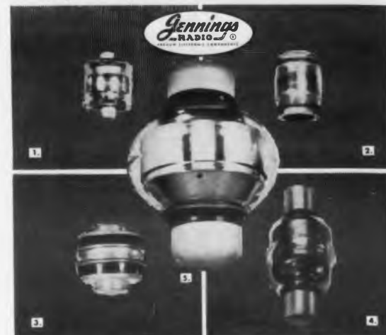
1. JCSL 1000 mmfd.; 3 KV; 42 amps rms 2. JCS 1000 mmfd.; 7.5, 10, 12 KV; 42 amps rms 3. MC-1 1000 mmfd.; 10, 15 KV; 75 amps rms 4. MC 1000 mmfd.; 10, 15, 20 KV; 120 amps rms 5. MLC 1000 mmfd.; 25, 30 KV; 120 amps rms 6. MMHC 1000 mmfd.; 35, 40, 45 KV; 125 amps rms
