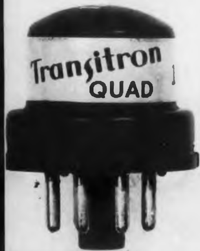
Fig. 2. The diodes are available in matched quads or pairs mounted in either octal bases (top) or 7-pin miniature bases (bottom).
