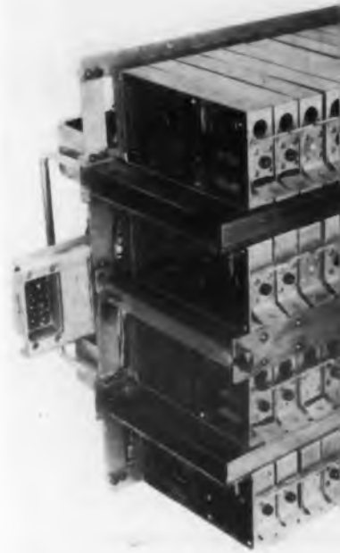
Fig. 2. There are three racks like this one supporting 80 plug-in circuit packages each.
