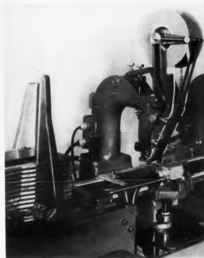
"Belted" resistors are running out of the spool at the top and being inserted into 5" x 8" printed-wired circuit boards by this United Shoe Machinery Corporation experimental machine.
