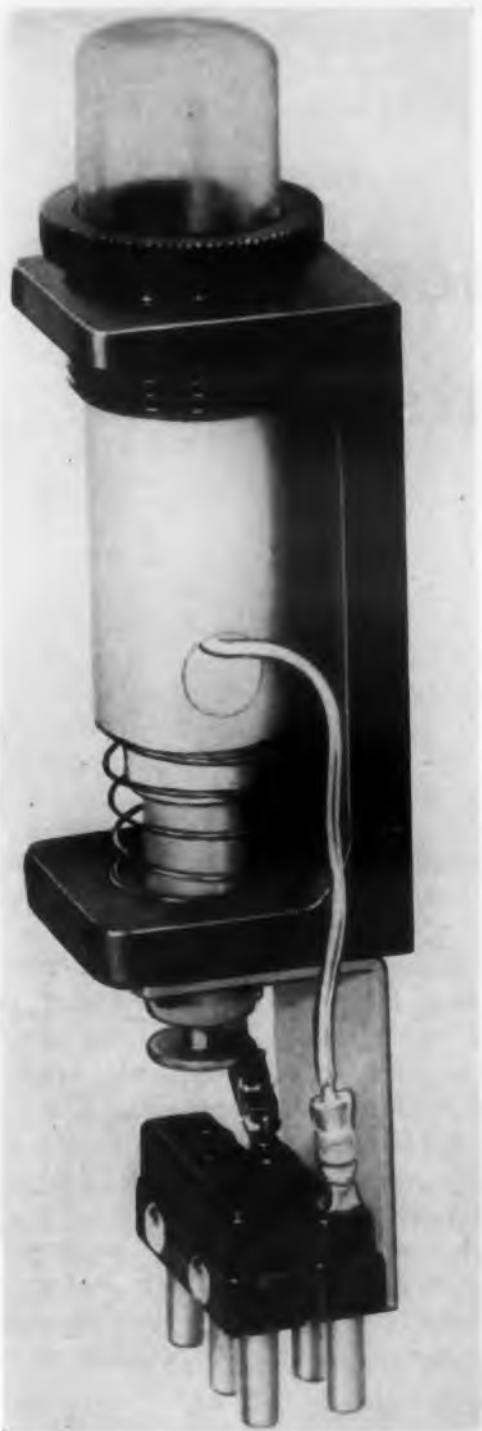
Switch-life is about 1,000,000 operations.
