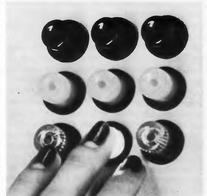
These switches can be mounted on one-inch centers.
