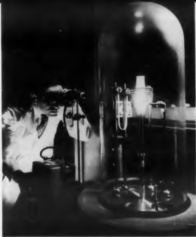
Titanium is being purified by the "cage zone refining" process in which it forms its own crucible.
