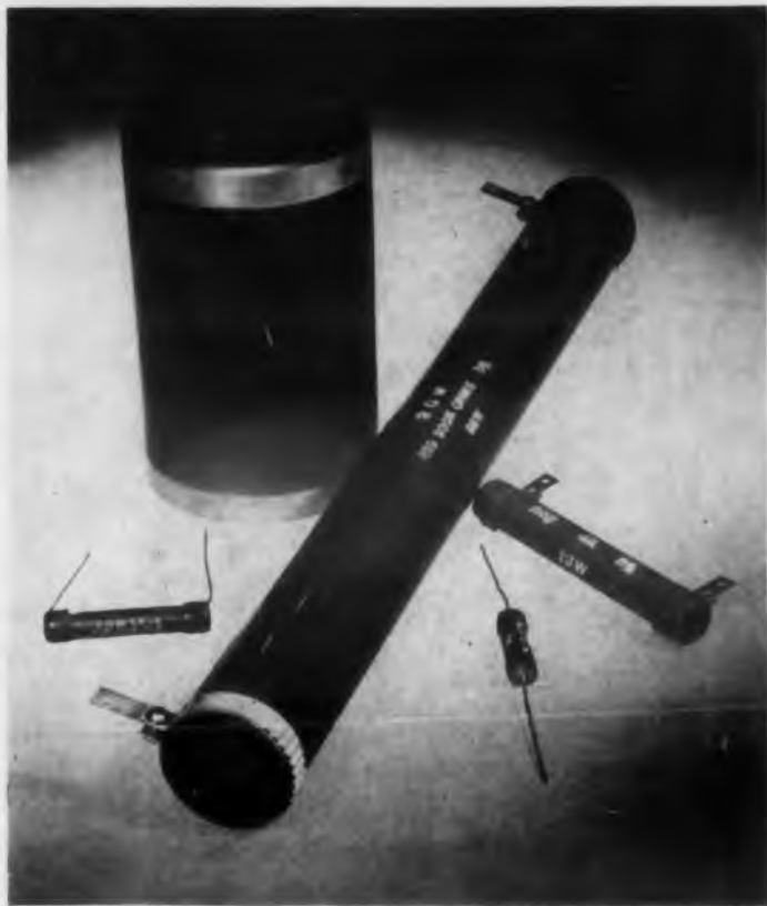
Electrically conductive metallic oxides bonded to glass tubing or rods make excellent resistors.
