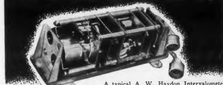
A typical A. W. Haydon Intervalometer which supplies precision pulses.
