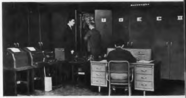
UDEC II, a complex pulse system. The giant Burroughs Unitized Digital Electronic Computer is built entirely from Burroughs Pulse Units connected together with standard cables.
