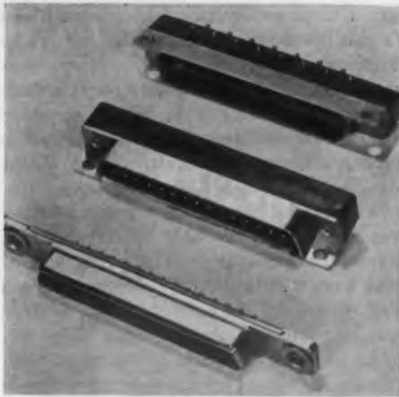
Fig. 6. New printed-circuit connector. Either male or female half can be dip-soldered to the board.
