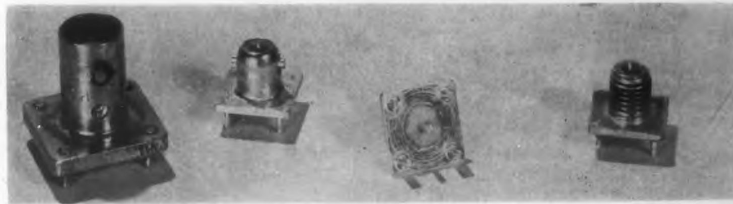
Fig. 5. Types BNC, MB and SM printed-circuit receptacles (l to r) for dip-soldering.
