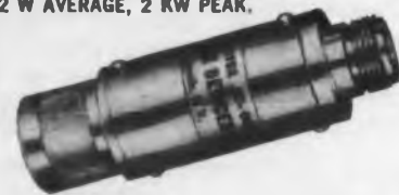
AT-60: ATTENUATOR PAD, DC TO 3000 MC. 2 W AVERAGE, 2 KW PEAK.
