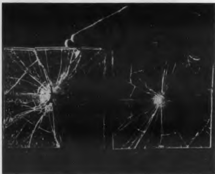
Fig. 1. After a few minutes at 375 F the plastic interlayer in conventional safety glass softens, bubbles and oozes out the panel edges, robbing the laminate of shatter-resistance. Panels based on Silastic Type K Interlayer, however, remains clear and shatterproof even after hours at 375 F.
