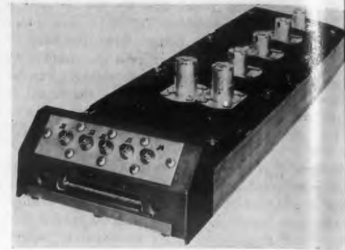
Fig. 8. A "packaged" printed-wiring assembly where complete shielding was required.
