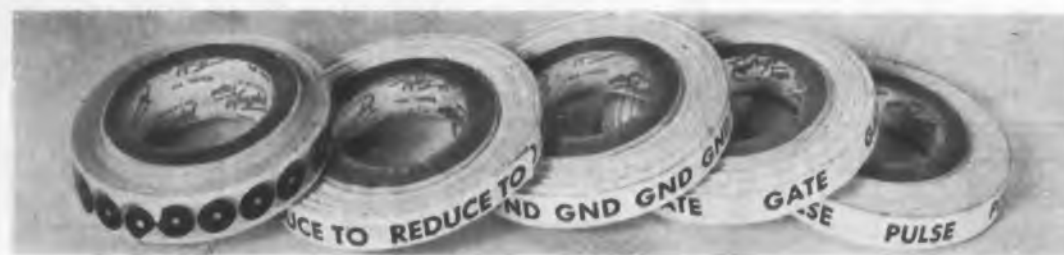
Fig. 1. Use of tapes saves time in laying out printed circuit board.
