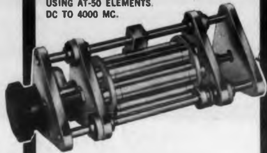
AT-50: ATTENUATOR PAD, DC TO 4000 MC. 1 W AVERAGE, 1 KW PEAK.
