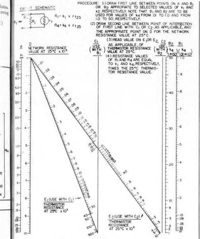
**Nomogram** for selecting values of  $R_t$  and  $R_t$  in the two-resistor network shown.
