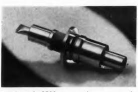
Machlett Laboratories announces the availability of a new ceramic UHF medium-mu triode designed primarily for use in grounded-grid cavity circuits as a plate-pulsed oscillator at frequencies up to approximately 4000 megacycles per second. This new tube also finds application as a radio-frequency power amplifier, continuous wave oscillator or frequency multiplier at frequencies to ap-
