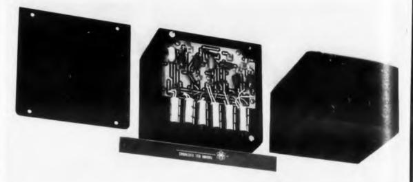
**Cooled to 225 C** by ram air, this amplifier-decoder is one-third the size of its prototype. The i-f strip exposed above has 75 db gain, measures  $1/2 \times 4-1/8 \times 3-3/4$  in.
