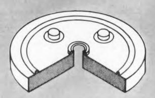
conductive plastic potentiometer element. The raised ring is conductive throughout its cross section and circumference except for the short section between terminals. Rear ball bearing and wiper contacts are also shown.
