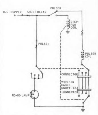
Fig. 2. Simplified drawing of open locater.
