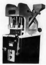
Mini-Jector 70VC95 is a precision injection molder for intricate parts requiring inserts a loose cores. It handles 0.33 to 1.5 oz parts and all thermoplastics, including Nylon. Maximum injecting pressure is about 30,000 lb.
