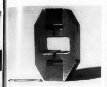
Fig. 4. Pole-piece design, showing detail of special silicon steel extrusions.
