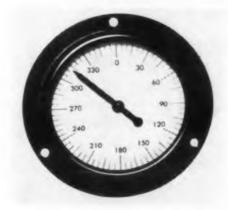
Using a dc synchro and a potentiometer transmitter, this remote readout system reads valve flapper and shaft angles through 360 deg. Accurate to 0.5%, it operates from 28 v dc and requires less than 0.1 w.
