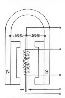
Fig. 1. Basic polar relay construction.
