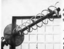
A very broadband antenna which easily covers the 2Kmc telemetry band.
