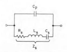
Fig. 2. Equivalent circuit of quartz crystal.
