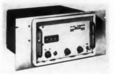
Measuring ac and dc voltage ratios from 01 1 in direct numerical values, model 1594 digital ratiometer has a full scale accuracy of ±0.19 Inputs range from 0 to 6 v dc and 0 to 6.3 v aca 400 cps. Reference input impedance for both and de ratios is 1 K.
