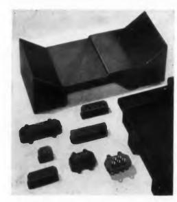
**DIALL F8-6** withstands prolonged exposure up to 500°F. At this temperature it retains a flexural strength of 1800 psi, a compressive strength of 6000 psi, and a tensile of 4300 psi. Substantially greater strengths at lower temperatures. An asbestos-filled, Diallyl Iso-Phthalate compound, it has succeeded where the best Silicone materials failed.
