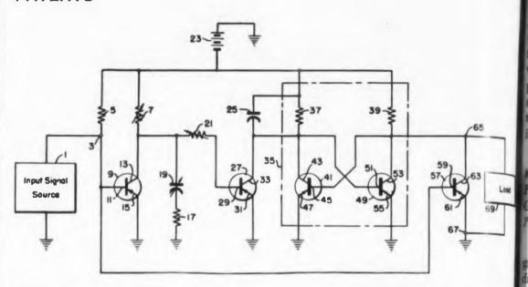
Static Time Delay Circuit
