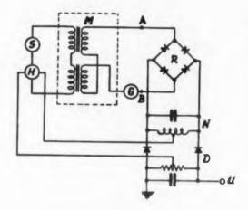
former primary contains signal source S and auxiliary generator H.
