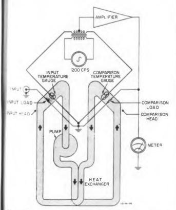
Fig. The series operation of the oil flow guarantees equal flow rates over both sensing elements.
