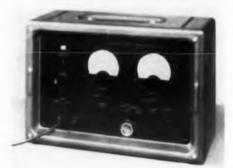
Type B-731A meter may be used for JAV MIL vibration tests on electronic components. permits remote measurement of vibration distances from 50 µin. to 0.5 in. and vibration rate from 1 cps to 10 kc. Accurate to 2%, the unit has a noncontacting probe and can measure to dilation and eccentricity of rotating parts.
