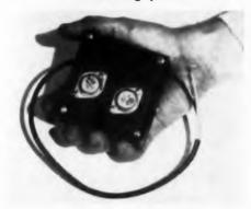
There are no moving parts or vibrators in this Corp., Des rugged power supply. Converting battery to B 1 Segund coltages with 80% efficiency, the unit has 0.05% output ripple and 0.3 v rms input ripple. It is VICE CARD \$5 in. sq and 1.7 in. high. Models TPS-1 and TPS-2 have outputs of 100 ma, 150 v and 200 ma, 250 v, respectively. Inputs are 12 and 24 v. P. R. Mallory & Co., Inc., Vibrator Div., Dept. ED. DuQuoin, Ill.
