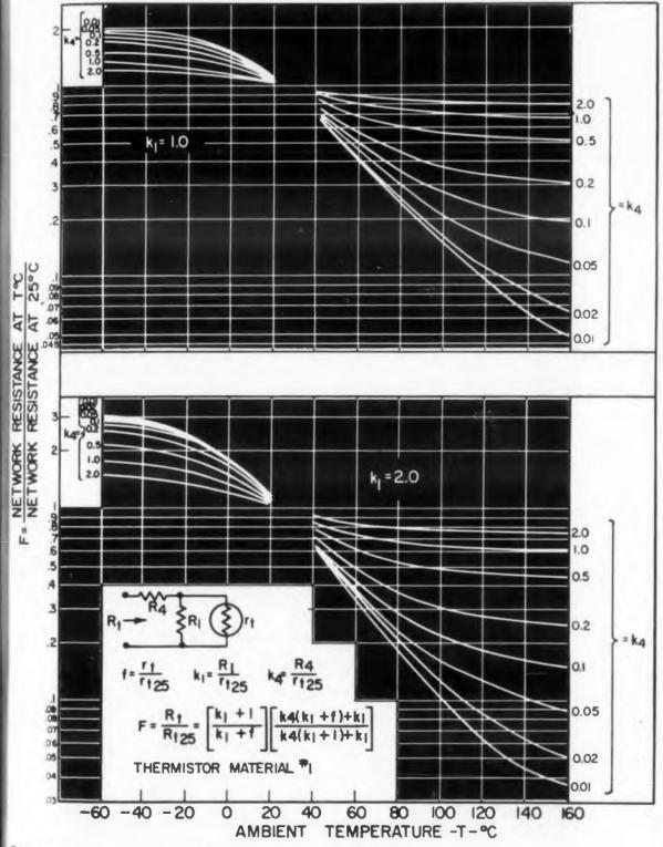
Common thermistor materials applicable are: Carborundum Carp.—type H; Fenwal Electronics—type No. 1; G. E.-Carbo Carborum—type Grade 1; Keystone Carbon—type 97; Thermistor Carp. of America (Gulton)—type D; Victory Engrg. Corp.—
