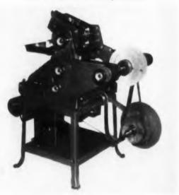
Designed expressly for diodes, this lead straightening and taping machine automatically reel packs axial lead components. It is adjustable for a variety of body lengths and diameters and can be adapted to lead or body taping.
