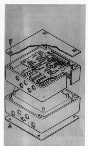
Fig. 1. Cutaway of amplifier-decoder. Solid packaging assures freedom from vibrational ills. Tubes are scoured by forced convection through holes in the bottom and top of the unit.
