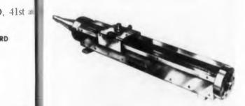
Slotted line type 1026 has a residual vswr clow 1.01 and less than 1.005 rated error in elected signal. Important outer conductor surces are hand scraped to fine tolerance. The ner conductor is supported by compensated electric pins. The unit is furnished in 20, 40, 1, 80, and 130 in. lengths and comes in standal impedances from 50 to 75 ohms. It may be red with tapered reducers for measurements 16-1 in., 3-1/8 in., 1-5/8 in., and type Noaxial transmission lines.
