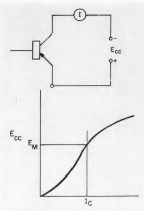
Fig. 1. Common emitter configuration. The voltage  $E_m$  is called the rated maximum. This is the collector voltage when some arbitary value of current is reached on the knee of the  $V_c$ - $I_c$  curve.
