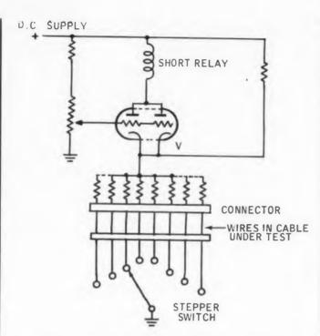
Fig. 1. Simplified drawing of short locater.
