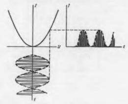
Fig. 26. Waveforms at the input and output of a beat detector.
