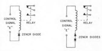
**Fig. 2.** (left) For dc circuits, a single zener diode can simplify relay speedup.
