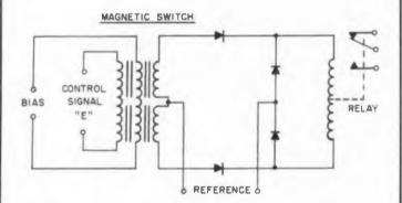
**Fig. 1.** Magnetic switches can speed up relays, but they're bulky and temperature sensitive.
