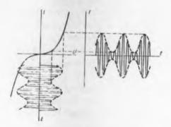
Fig. 29. The nonlinear characteristic  $l = kU^3$  is not suitable for detection since the oscillation remains symmetrical about the time axis.
