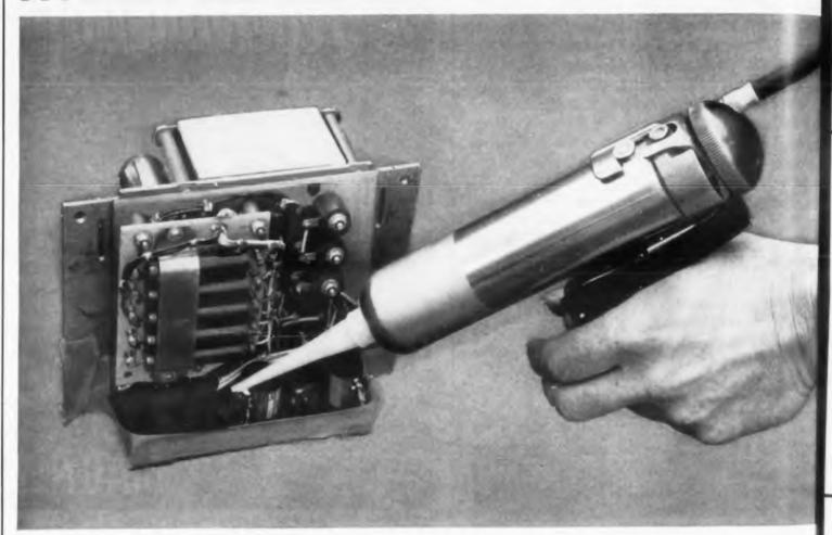
High impedance circuits in Northrop's Snark missile are coated with Silastic RTV for protection against moisture and vibration at temperature extremes. Silastic RTV is easy to apply . . . vulcanizes at room temperature.
