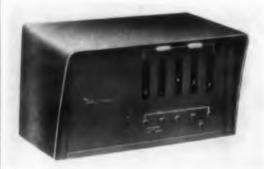
With a single zero, this decimal electronic mter indicates true positive and negative abers Counting to  $\pm 99999$ , it operates at s up to 50 kc. Available with a buffer storage t the counter receives its input from a toele ric shaft to pulse converter which gentes 10 4 counts per shaft revolution.
