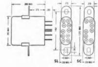
SL—dual coil latching relay. Operates on a 230 mw, 3 ms. pulse at 25° C. Permanent magnet latch locks the armature in either position.
