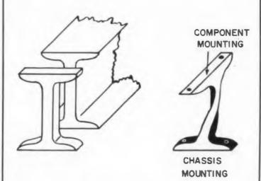
A twisted aluminum I-section for a sturdy bracket.
