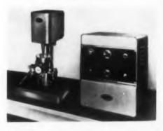
Model 2-335 ultrasonic impact grinder of slices, drills, and trepans regular and irregular shapes. It handles semiconductors, ceramo ferrites, carbides, metals, jewels, and other to brittle materials. Its magnetostrictive traducer permits a 100% duty cycle.
