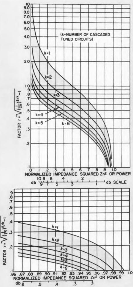
Fig. 3. Curves of r as a function of  $Z_N^2$  or power for various values of k. Region around  $Z_N^2$  value of 1 has been redrawn on an expanded scale.
