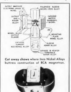
port, provides high strength, corrosion resistance and low magnetic permeability certified not to exceed 1.1 in a field of 0.5 oersted. Monel "403" alloy has the dimensional stability needed to maintain the cathode centered in the anode over many heating cycles. It also offers easy machining and retains its non-magnetic characteristics after cold-working and forming so that highstrength parts can be assembled without annealing.
