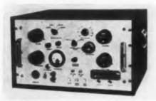
This tester checks out L-band airborne transponders built to ARINC characteristics 532B and ANDB (AMB) 2.3 NAIB. Frequency range is 950 to 1220 mc; repetition rate, 15 to 2000; pulse spacing, 1 to 30 µsec.
