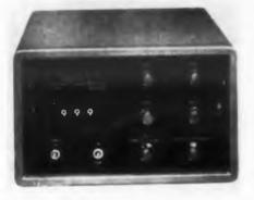
The DTI-2 digital torque indicator supplies an output proportional to horsepower. It is equipped with a slidewire which, when excites by the output of a tachometer generator, wis supply a strip chart recorder with direct horsepower readings. For 115 v, 60 cps ac operation the indicator has an accuracy of  $\pm 0.15\%$ . A constant voltage supply within the unit prevents from responding to line transients.
