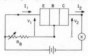
Fig. 1. Basic Circuit
