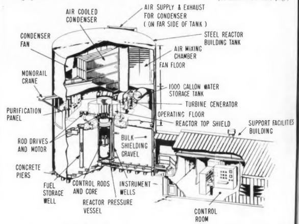
Easily transportable in cargo planes, this Argonne Low Power Reactor is destined for such remote stations as DEWline radar bases. It provides 200 kw of electricity, 400 kw of heat.
