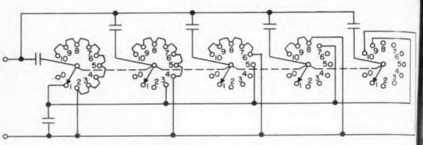
This decade capacitor doesn't open the circuit when it is switched from one value to the next.
