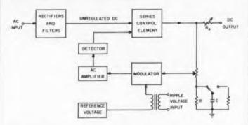
**Block diagram** of a typical regulated power supply with provision for increasing load regulation, introducing ripple, and creating transients.
