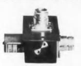
At right is a Tuner Assembly for matching a Marker Beacon Antenna which is mounted in a supersonic aircraft.
