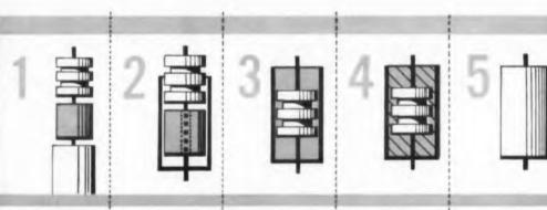
The "E-FORM" pellet and electronic component are inserted into the "E-CASE". in that order. The assembly is then subjected to heat, with a gentle pressure exerted on the component. The heat causes the pellet to liquefy and flow around the component. Further heating gels and then cures the epoxy. The result is a completely epoxy-encased unit, resistant to humidity, temperature variations and corrosive influences.
