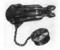
Weatherproof LR and MR connectors have clear and black anodic coating to resist corrosion and rubber glands and gland nuts to seal out noisture. Chain-attached caps seal unmated mits. Coupling threads and sizes are standard to MIL-C-5015.
