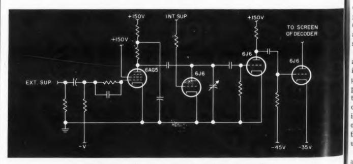
Fig. 2. Conventional suppression circuit, designed with tubes.
