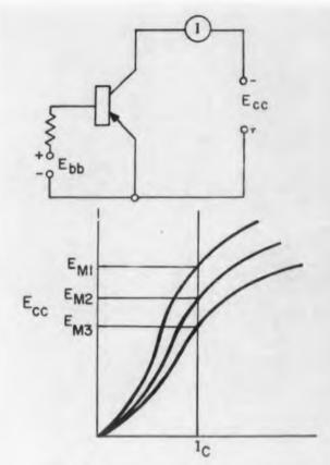
Fig. 2. A reverse bias is applied to the base-emitter junction. The voltage rating is 2 to 3 times than that obtained with base disconnected.
