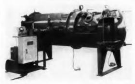
Type 742 inert gas welding machine is a proparts a duction unit for reactive materials such as zir-Maximu tonium, tantalum, and columbium. For manual r semiautomatic operation, it has dual welding ED, New positions with glove ports, sight glasses, autonatic welding shields, and lights. It has a high peed, high vacuum pumping system and an hert gas backfill system. In lengths from 6 ft, he units are 42 in. in diameter.
