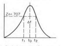
Fig. 1. Typical response of resonant circuit.
