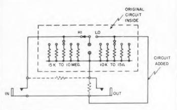
**Heath substitution box,** modified to serve as attenuator. The attenuation equals the "Lo" resistance divided by the sum of the "Lo" and "Hi."
