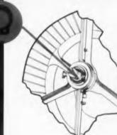
Fraser and Johnston Co., San Francisco, Calif., uses a Series 5555 Grip ring\* to secure the fan shaft and speed assembly of its furnace blowers. The ring eliminates a collar and set screw for savings of \$180/M on materials, \$80/M on assembly time—a total of \$260 per 1000 units.
