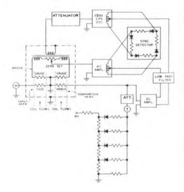
Fig. 1. Circuit diagram of the rf power meter.
