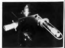
This coaxial filter covers the 2 to 4 kmc range. Its single micrometer knob is set to reject any frequency in this range to the extent of about 30 db with less than 1 lb loss at nonresonant frequencies.
