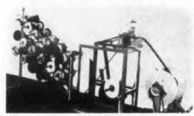
With this automatic cable machine, any type of Zippertubing cable can be made at speeds up to 900 ft an hour. Easily operated, the unit eliminates an extruder. It makes cables of up to 108 conductors and from 3/8 to 2-1/2 in. in diameter.
