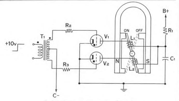
Fig. 2. Modified polar relay interconnected to a firing circuit.
