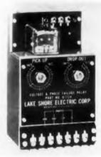
This differential voltage sensing operate relay protects radar gear, micro-C. Ther wave relay systems, and other quipment. Its control range is 70 to 100% of rated voltage for both D, 1521 dropout and pickup with a minimum 1 v differential. Dc ranges re 6 to 49 v and 50 to 250 v; ac ranges are 1 and 3 phase, 3 and 4
