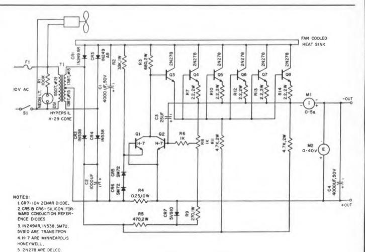
Fig. 1. Schematic of power supply.
