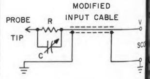
**Modified low capacitance probe** provides less nal attenuation with same capacitance. R = twice input resistance of the scope. C is a 2 to 12 unit mer.
