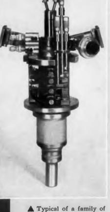
high-power klystrons under development is this 1-KW CW power output tube (solenoid and cover removed) which tunes over a 1000 mc range at X-band, with 40 db gain. All tubes in this family are of rugged, metal-ceramic construction to meet performance standards of military specifications, and employ an extremely long-life, singleknob tuner. Other designs include high-power tubes for L, S and X bands.
