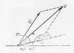
Fig. 28. Vectorial addition of two voltages of unequal frequencies.
