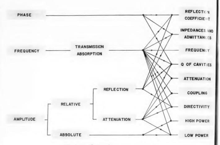
Fig. 1. Classification of microwave measurements
