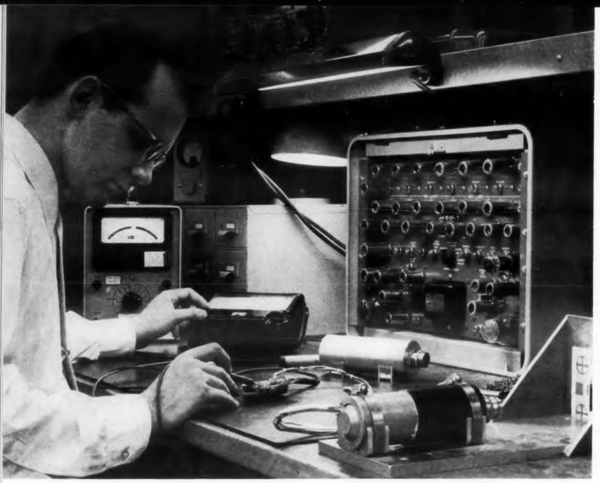
A MISSILE AND TELEVISION INDUSTRY FIRST. Lockheed-developed, miniaturized TV cameras, designed for both government and commercial use. Only 6 inches long and 2½ inches in diameter, tiny cameras extend man's vision into the unexplored. Unmanned lunar probes to the far side of the moon; lunar landings; monitoring interiors of manned spacecraft and remote TV coverage of on-the-spot happenings on a scope never before possible are some of the uses foreseen for the cameras.
