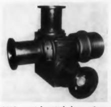
Type 1038 coaxial switch has a 0 to 450 m frequency range and a vswr under 1.05. It is designed for 6-1/8 in. coaxial transmission line and has about the same cw power rating as they do. It comes in motor and manually operated models.
