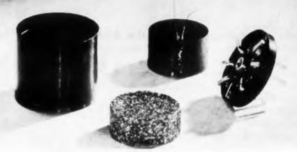
**Fig. 1.** From left to right are the shell, the premetered pellet, the component and the header.
