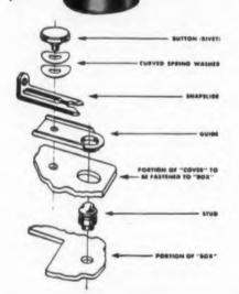
This positive, quick-action fastener was originally developed to hold airborne equipment with security - even under severe stress and shock of carrier-based aircraft operations—and yet permit equipment replacement in a matter of seconds.
