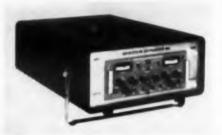
Model 940 dual channel amplifiers are designed to drive the company's 102 and 120 gd vanometers. Frequency response is dc to 10 kd  $\pm 1$  db; input impedance, 1 meg constant; input sensitivity,  $\pm 1$  to  $\pm 100$  v for full scale output The unit can provide  $\pm 10$  v at 200 ma.
