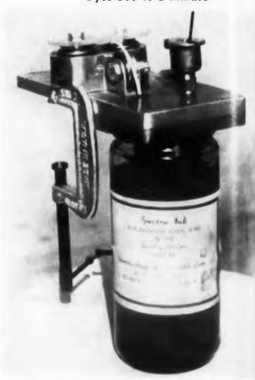
Spectra-Coder model 701 dyes 500 ft of a minute. It handles any vinyl insulated where, and can be used with Spectra-Ink or other instant drying ink.
