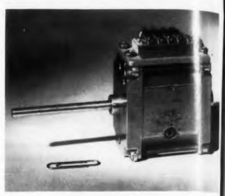
Fig. 3. Assembled highspeed magnetic actuator.
