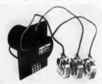
Driven by a single phase hysteresis motor, the 105A sampling switch has three poles, each with 30 shorting or 15 nonshorting channels at 1 rps. No brush force or phase adjustments are needed to replace the rotor and brush assembly. The unit has multipin connectors.
