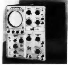
A fast-rise, cathode ray oscilloscope, type 543 handles do to 30 mc. For versatility, nine plug-in preamplifiers are available. Sweep range is 0.02 usec per cm to 15 sec per cm; accelerating potential is 10 kv. The built-in voltage calibrator has 18 outputs from 0.2 mv to 100 v peak-topeak. The unit has sweep magnifications of 2, 5, 10, 20, 50, and 100 times. A single knob controls 24 direct-reading calibrated sweep rates.
