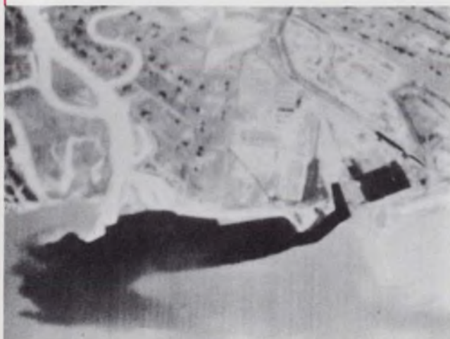
Infrared scan (left) shows the hot water discharge from a power plant into a waterway. After conversion of the gray scale into discrete colors (purple is the hottest and
