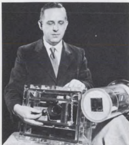
Underwater camera system developed by NASA. Russell J. Jirberg adjusts the timing mechanism that he designed for the system.
