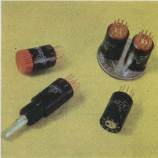
Miniature rotary switches for PC-board mounting include (upper left and clockwise) AMP 642-1 series units, the Minelco SW 37 and 67, the Edison, Daven Dip-switches and the Grayhill Series 75. Other rotary-switch manufacturers are turning out similar types in an almost endless flow.
