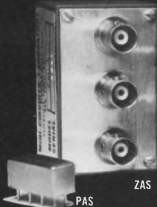
The PAS/ZAS series of electronic attenuators enable attenuation control of rf signals with a maximum of only 20 mA of control current. Due to the specific properties of these attenuators, for a single frequency input all harmonics even and odd order are virtually eliminated at the output. As a consequence, the PAS/ZAS intercept point is greater than +50 dBm. The series covers a very broad frequency range from 1-450 MHz.
