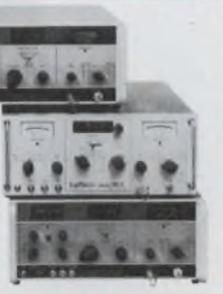
LogiMetrics provides the industry's most complete line of solid state signal generators, all of which are equipped with digital frequency readout. The signal generators cover the range of 50 kHz to 520 MHz with integral counters and leveled outputs. A precision attenuator allows the power to be varied from +22 dBm (10 W RMS) to -127 dBm (0.1  $\mu$ W RMS) into 50 ohms.
