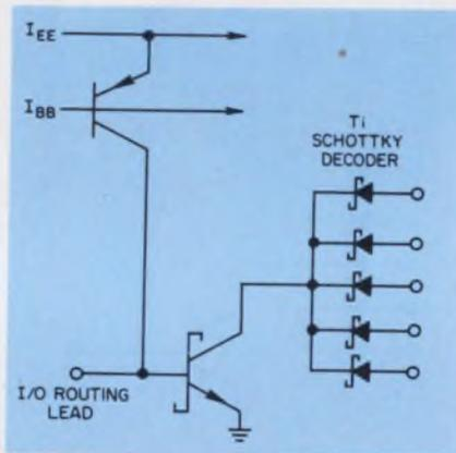
Multiple inputs and outputs are possible with a C<sup>3</sup>L NAND gate. The I/O routing lead connects to the collectors of driving gates.
