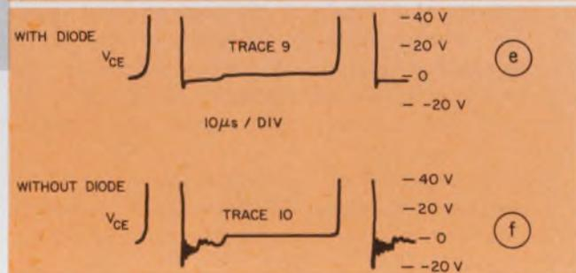
3e, 3f) show the collector-emitter voltage at the end of the retrace with and without the damper diode. In Fig. 3e the voltage is clamped to the diode forward voltage and in Fig. 3f to  $BV_{EBO}$ .
