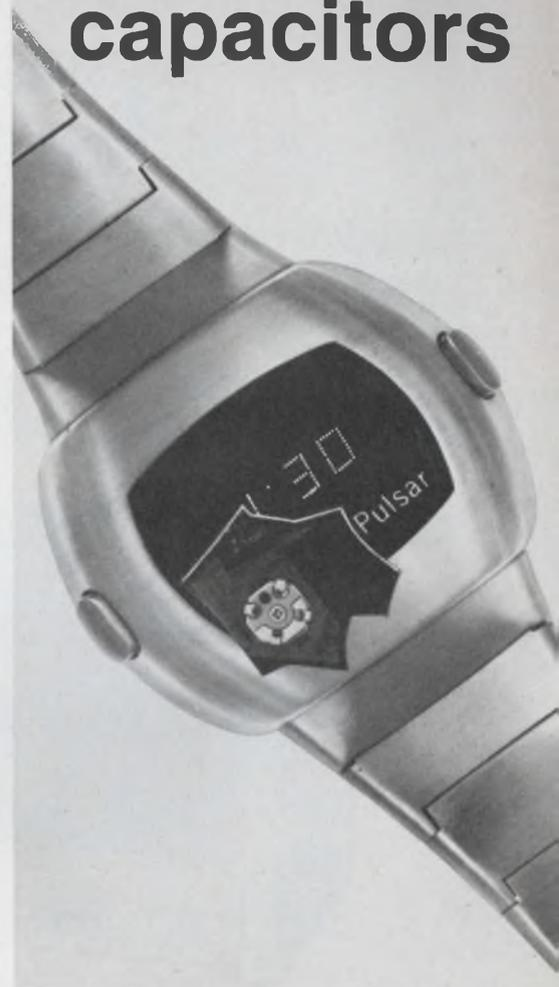
Tucked in the corner of this Pulsar Watch is a miniature capacitor which is used to trim the crystal. This Thin-Trim capacitor is one of our 9410 series, has an adjustment range of 7 to 45 pf., and is .200" x .200" x .050" thick. The Thin-Trim concept provides a variable device to replace fixed tuning techniques and cut-and-try methods of adjustment. Thin-Trim capacitors are available in a variety of lead configurations making them very easy to mount.
