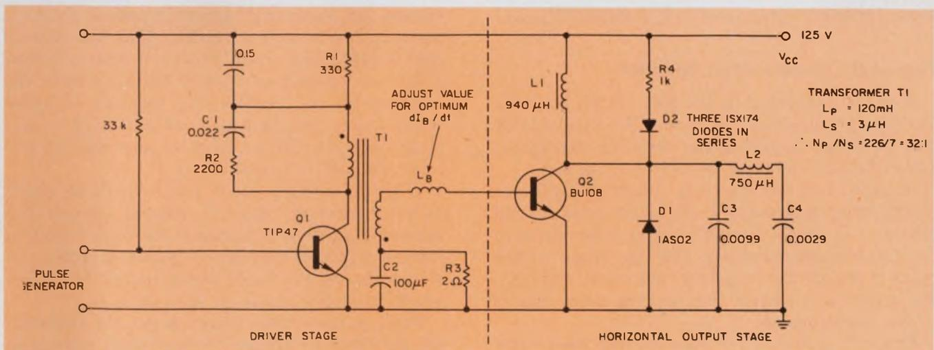
1. A test circuit can simulate the horizontal output stage of most CRT display systems. This can help evaluate the
