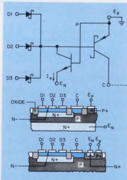
Schottky transistor logic gate (top) uses Schottky diodes and a pnp (m for metal) transistor to get a five-fold improvement in power delay over conventional I<sup>2</sup>L. Practical STL structures can have either vertical (middle) or lateral (bottom) supply injection.
