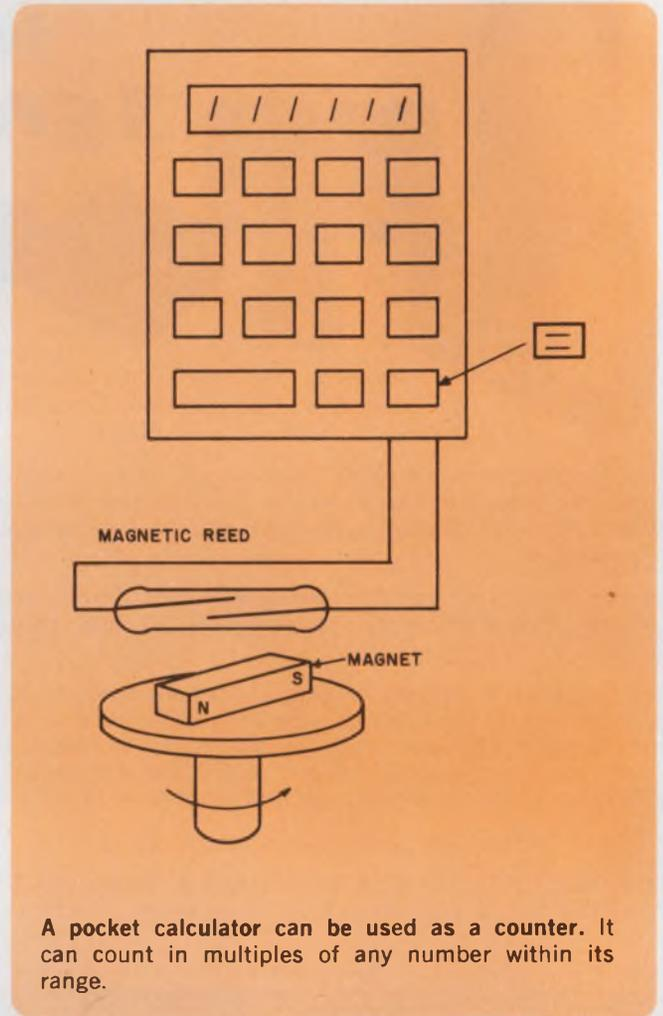
A pocket calculator can be used as a counter. It can count in multiples of any number within its range.
