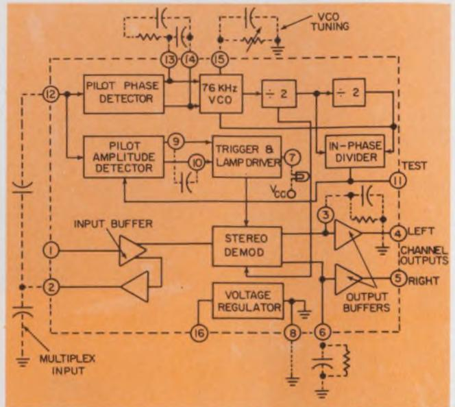
One phase-lock device bucking the trend to specialization is a micropower CMOS unit developed by RCA (CD4046) and second-sourced by Motorola (MC14046). It has been designed for a number of applications, including FM modulation and demodulation, frequency synthesis, data synchronization, tone decoding and motor-speed controls.
