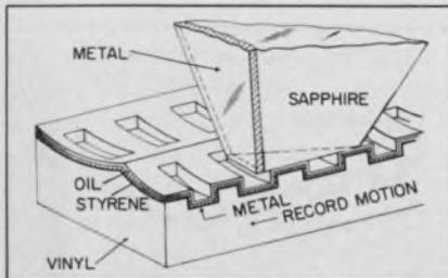
Capacitance pickup detects variations in the width and separation of slots in record groove that contains recorded information.
