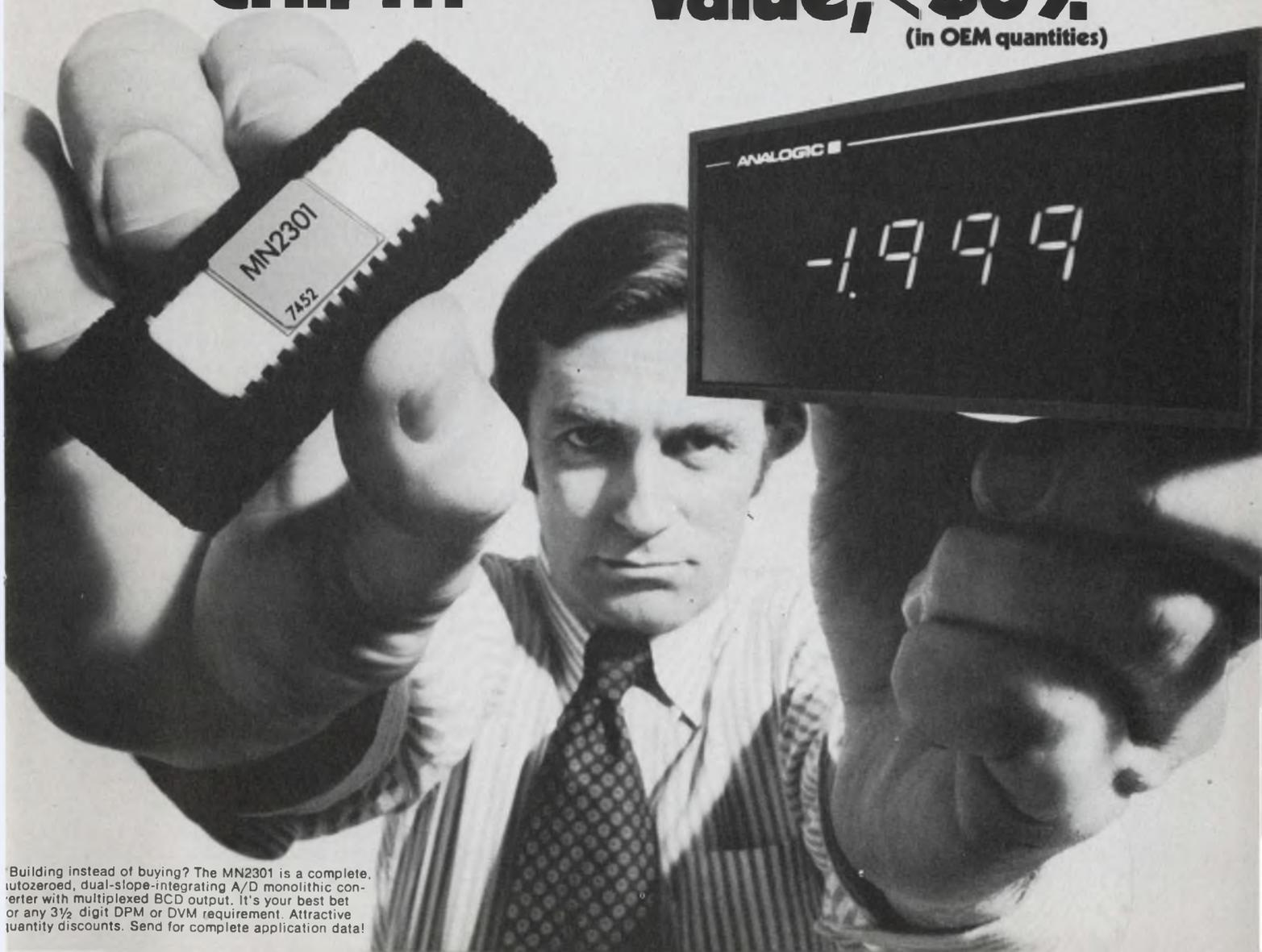
Building instead of buying? The MN2301 is a complete, autozeroed, dual-slope-integrating A/D monolithic converter with multiplexed BCD output. It's your best bet for any 3½ digit DPM or DVM requirement. Attractive quantity discounts. Send for complete application data!
