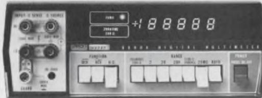
If our Model 8800A is not the perfect 0.005% bench DMM, it's close. You won't find any weak points. It's strong in every area: ■ 1 μV resolution with 0.01% accuracy for 90 days over a temperature span of 18° to 28°C.
