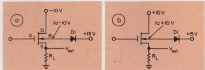
5. The back-to-back diodes don't significantly affect body-to-source or body-to-drain voltage, even though the analog input may be  $-10$  V (a) or  $+10$  V (b). For both cases the voltages referenced to body are both about  $0$  V.
