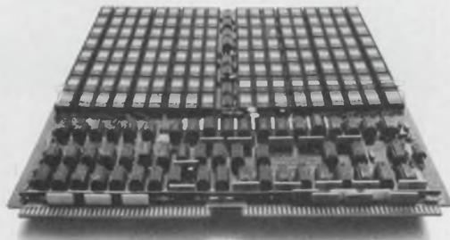
It's all of those and more, much more. It's our new Micromem 3400N — a 32K x 16 or 18 bit memory system using our own SEMI 4402, 4K STATIC RAM components . . . the only production 4K STATIC RAM's available today. The 4402 is fast, with a worst case access time of 200 nsec. And . . . it's second-sourced, of course!
