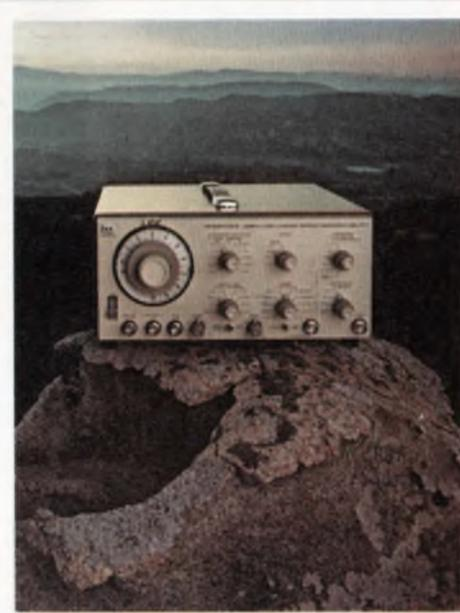
constant width setability from 30 ns to 10 milliseconds, and full offset and mode flexibility. The generator's fully-calibrated attenuator gives you 15-volt unipolar pulses into high impedance loads, particularly useful for testing MOS, or millivolt pulses down to 1.5 mv.
