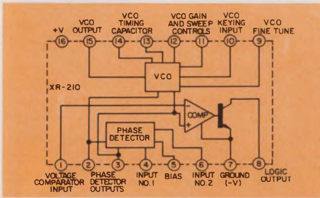
1. Designed for data communications, this Exar 210 phase-locked-loop IC is used in modems for FSK demodulation and for tone decoding.
