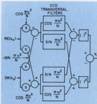
An analog Fourier transformer can be built by use of charge-coupled devices as transversal filters. The technique shown employs a sliding chirp Z transform for periodic waveforms and stationary signals. A practical system has been built to generate a 500-point transform.
