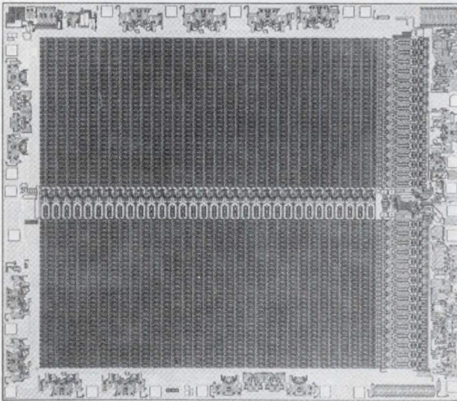
**Aiming for ECL-oriented systems, Intel's latest 4096-bit MOS RAM has access time of less than 80 ns. The ECL-compatible chip employs charge-pump techniques to obtain operational features of static units.**
