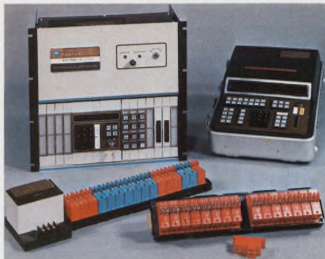
Features often associated with minis combine with the ease-of-use of other programmable controllers in the Eptak industrial-control system from Eagle Signal. The system uses the 8080 \mu P.
