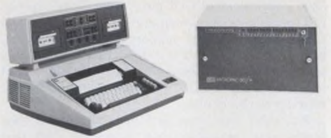
One of the first development systems to use the 8080, Process Computer Systems' Micropac 80/A simplifies the design of controllers for industrial equipment.
