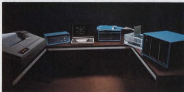
The most advanced development system for micros, Intel's MDS (microcomputer development system), features in-circuit emulation. The capability permits early fault and error isolation in system prototypes. MDS includes floppy-disc storage and a CRT terminal, and allows the setting of breakpoints symbolically.
