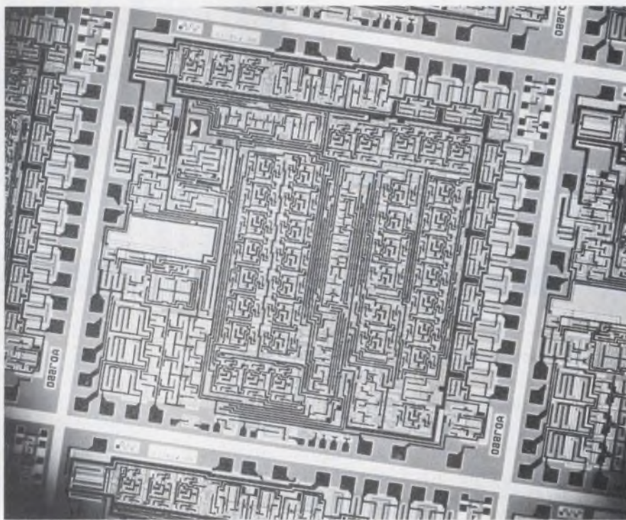
Analog Devices' 13-bit CMOS ADC uses a quad-slope conversion technique.
