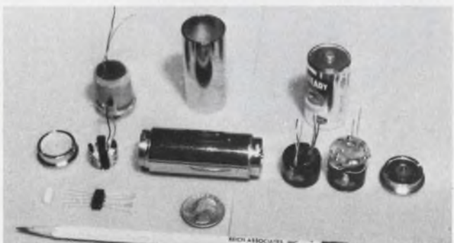
Highly compact dc-to-dc power supplies, such as this 16 kV at 1 \mu A unit produced by Reich Associates, can operate from a 1.5-V source.
