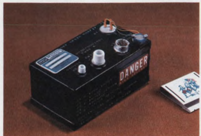
Small, modular power supplies, such as this 6-kV unit made by the Capatron Div. of Amp, offer multiple outputs that can operate at temperatures of 100 C.
