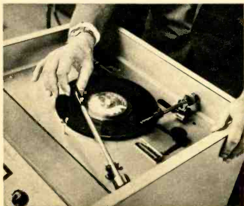
Record/player unit for the broadcast industry turns a 9-in. disc at 2 rpm. It is designed to make recording of an entire day's broadcasts.
