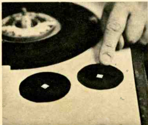
Home applications envisioned by inventor Robert Wagner include recorder/player the size of pack of cigarettes to accept 2-in. discs like these.
