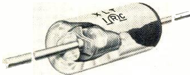
Fig. 1. Cutaway view of a typical glass-sealed precision resistor made by IRC for use in the "Minuteman" guided missile.
