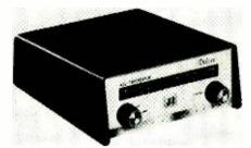
The Model CR1-J is designed for local area and suburban use and has one transistor in the oscillator circuit and a mixer diode. The CR2-J converter has two transistors--one each in the oscillator timer and i.f. amplifier stage-and is designed for fringe area applications.
