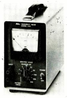
THE Waters Model 343 frequency meter is a completely transistorized portable device for the measurement of the frequency of repetitive waveforms in the range 20 cps to 50,000 cps. Readout is an analog indication on a  $3\frac{3}{2}$ " d'Arsonval meter. The meter is calibrated from 0 to 100 and switched multipliers of 1, 2, 5, 10, 20, 50, 100, 200, and 500 are provided. Accuracy is better than  $\pm 2\%$  of full scale.
