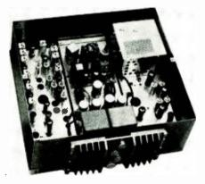
are in production. The transmitter, receiver, and power supply are assembled on separate chassis strips with special attention being given to cool operation and easy maintenance. The chassis is wired for phig-in addition of continuous tone squetch. Standby drain is 2.5 amps.
