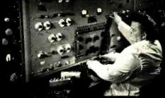
Voltmeter being calibrated on the RCA AC Voltage and Current Standard.
