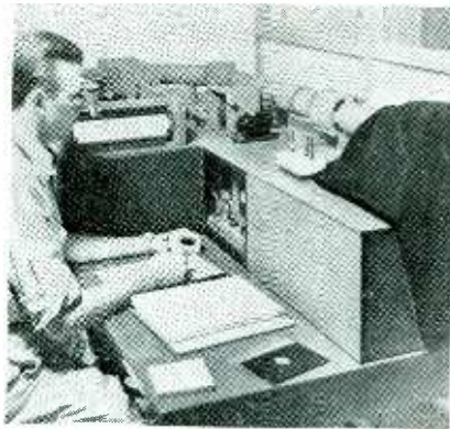
An operator makes a test with the G-E spectrophotometer. The instrument measures and records curves of over two million shades of color
