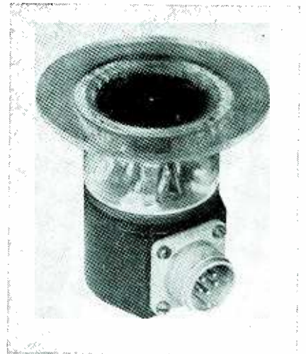
Pickup with plastic hood, facilitating mounting over the glass face of an instrument
