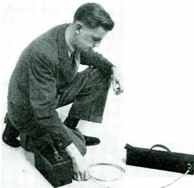
Typical counting apparatus. The G-M tube is mounted in the probe unit at the right, which plugs into the amplifier and counter
