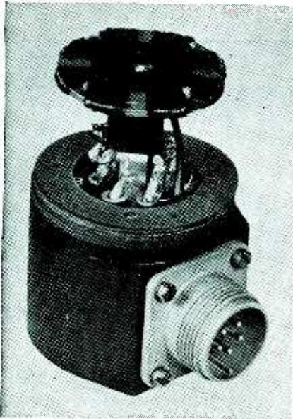
Electronic position pickup, showing two-phase winding on a circular disc mechanically linked to a piezoelectric crystal. The disc is mounted in close proximity to an instrument pointer equipped with a small permanent magnet. There are no moving parts
