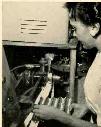
Belt pulls plates to vacuum pickup. Paper is most economical belt material
