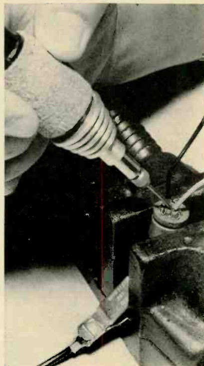
Use of single-electrode iron. Other lead of transformer is clipped to metal fixture plugged into connector
