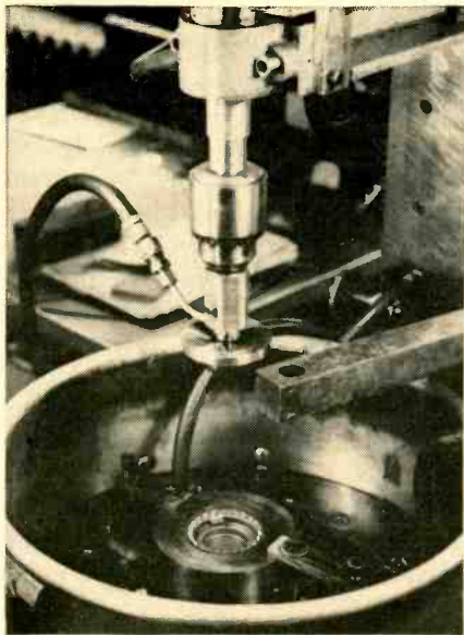
Tool and die mounted in spark machine
