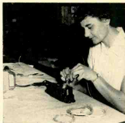
Two-electrode resistance iron used to solder connector held in bench vise
