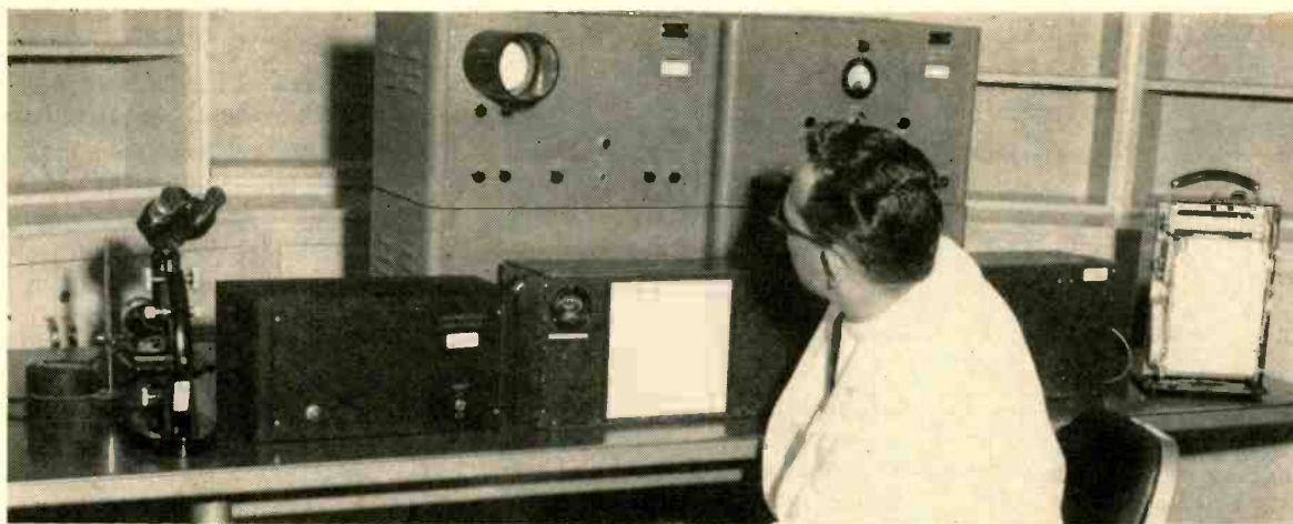
Doctor adjusts video clipping level control for maximum contrast. Ink recorder at extreme right provides densograms
