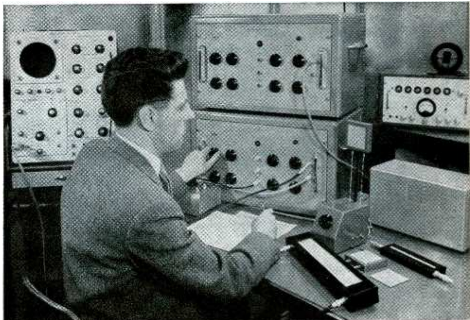
Operator prepares to display pulse waveforms on the small square screen
