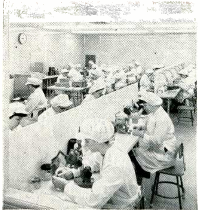
Precision trimmer potentiometers are assembled in "clean room"
