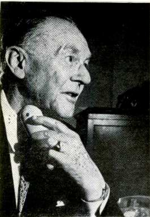
Electronic larynx developed by Bell Labs weighs only seven ounces, closely resembles a modern electric shaver. Power is supplied by Mallory 5.4-v mercury batteries
