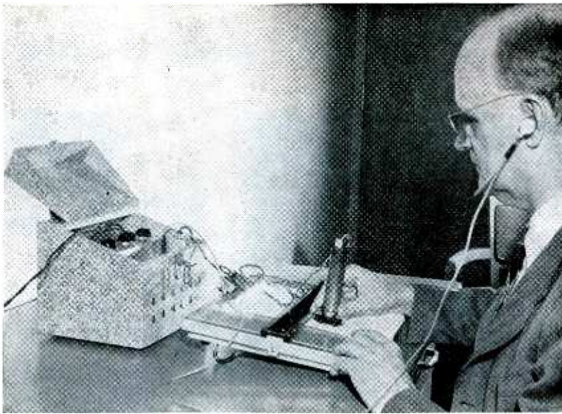
By passing photoelectric stylus of Battelle Memorial Institute's reader along a line of print, blind subject is presented with aural representation of letter scanned. Subjects have learned to read at 15 words a minute 7
