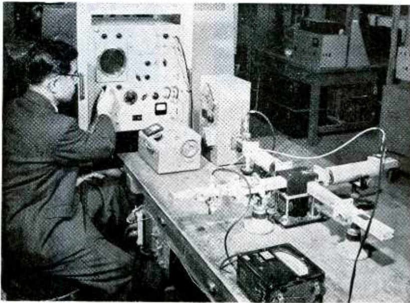
Author measures varactor quality (variation of capacitance with bias) with 6-Gc broadband impedance display unit
