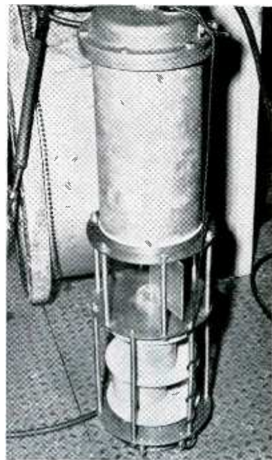
Pod parts are (from top) digitizer, direction sensor and rotor
