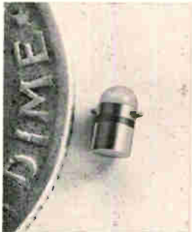
Figure 5. TIXL01 solid-state light source. Unit mounts directly in 1/16 in. printed circuit board.
