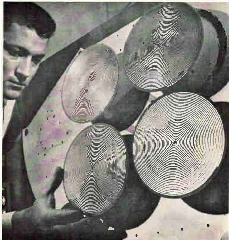
Antenna system consists of circularly polarized antennas in the form of Archimedean spirals, printed directly on epoxy boards. One transmitting antenna and three receiving antennas—azimuth and elevation measurements share a common antenna—shown by Westinghouse engineer, O. Lamar Bishop, are in the front of Gemini. Transmitter antenna and common receiver antenna are fixed, while the azimuth and elevation receiver antennas can be rotated.
