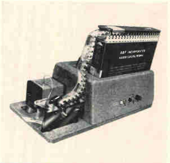
The compact AMP-TAPETRONIC* Pneumatic bench machine applies tape-mounted contacts to wires from size 10 to 26 AWG.
