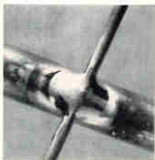
Cross weld between 0.005-in. diameter tungsten and 0.020-in. diameter nickel wires.
