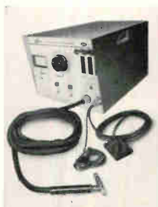
Repair welding of hermetically sealed relay case, using LINDE plasma needle arc torch.
