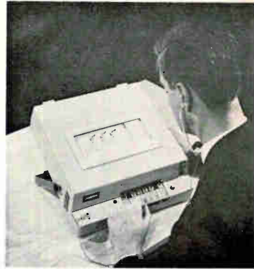
Ready for more? Brown Boveri teaching machine moves on to a new lesson segment or backtracks in both audio and visual channels depending on student's pushbutton answer to quiz.
