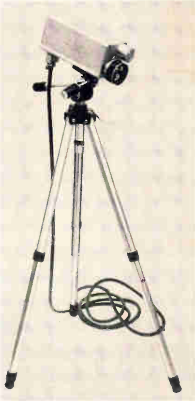
Light and colorful. CBS's new miniature color television camera uses the same color-wheel-and-vidicon technique proposed for network tv in the early 50's. Its size, weight, and price suit it to applications in medicine, on the battlefield and in space.
