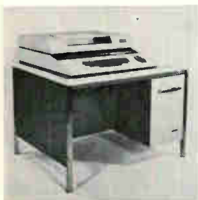
Data terminal EDX-1901 is for use in communications and data processing systems. The basic unit includes a keyboard, a page printer, a tape reader, and a tape reprocessor. It is designed for operation with the USASCI code and asynchronous operation at either 15 or 25 characters per second. General Dynamics, Electronics Division, P.O. Box 2566, Orlando, Fla. 32802 [425]
