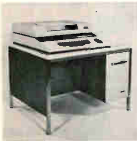
Data terminal EDX-1901 is for use in communications and data processing systems. The basic unit includes a keyboard, a page printer, a tape reader, and a tape reprocessor. It is designed for operation with the USASCII code and asynchronous operation at either 15 or 25 characters per second. General Dynamics, Electronics Division, P.D. Box 2566, Orlando, Fla. 32802 [425]
