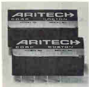
Sample and hold modules series SH-100 are for fast and medium speed data sampling and acquisition applications. They feature 0.01% accuracy, 50 nsec aperture time, 2 \mu sec acquisition time and a 1,000 megohm input impedance. Units are potted, contained in less than \frac{3}{8} cu in. and operate over a temperature range of 0 to 70°C. Aritech Corp., 130 Lincoln St., Brighton, Mass. [381]
