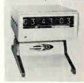
Time code reader model 8230 is designed to translate IRIG A, B, and E modulated time code formats in terms of BCD hours, minutes, and seconds without the need for switching or code plug removal. It will find use where data must be retrieved from magnetic tape recordings for access and identification during playback. Systron-Donner Corp., 888 Galindo St., Concord, Calif. [428]
