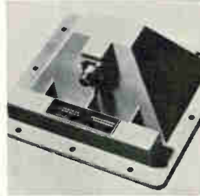
Radar altimeter antenna 0-1-34-04530 has metallic directors within its aperture to correct the E and H plane beam instead of a dielectric lens which is susceptible to shock, vibration and other environmental hazards. Unit operates at 4,300 \pm 50 Mhz, with a gain greater than 13 db and efficiency greater than 85%. Electronic Resources Inc., 4561 Colorado Blvd., Los Angeles [403]
