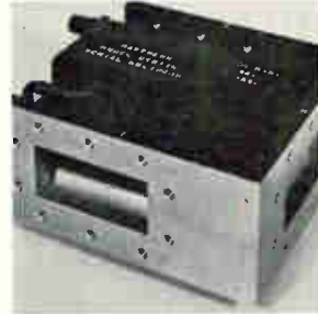
Waveguide junction circulator CSH116 is for industrial microwave heating uses. Operating at 2,450 Mhz, it can handle 10 kw c-w power with water-cooling or 5 kw without cooling. Minimum isolation is 20 db and insertion loss is 0.2 db maximum. Vswr is 1.20 maximum. It can be furnished with a dummy load at port-3 if required. Raytheon Co., Waltham, Mass. [407]
