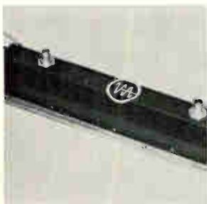
Cathode-pulsed twt VTC-5261J1 is for use as a driver or output tube in pulse-radar missile-guidance systems that operate between 5.4 and 5.9 Ghz. It produces more than 1 kw of peak output power at an 8% duty cycle from a package weighing 4.5 lbs and measures slightly more than 12 in. long, less than 3 in. high and 3 in. wide. Varian, 611 Hansen Way, Palo Alto, Calif. [401]
