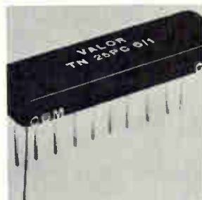
Lumped constant delay lines are low silhouette 5 to 200 nsec units for computer applications, radio and radar uses. They meet or exceed MIL-Standard 202 for moisture resistance, vibration, shock, humidity and life, and the basic requirements of MIL-D-23859. Temperature range is 55° to 125°C. Price ranges from $3.25 to $19.90. Valor Electronics Inc., Costa Mesa, Calif. [387]
