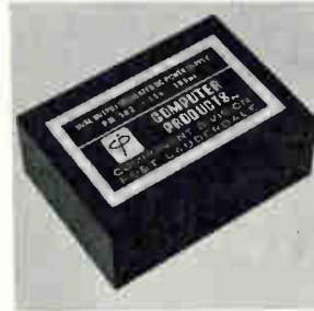
Dual output d-c regulated supply PM502 is for operational amplifier power source use. It operates directly from 115 v a-c \pm 10 v a-c, 50 to 400 hz, and supplies two regulated (line-load 0.02%) d-c outputs of \pm 15 v each delivering from 0 to 100 ma. Case size is 3.5 x 2.5 x 1.25 in. Weight is about 16 oz. Computer Products Inc., 2709 N. Dixie Highway, Ft. Lauderdale, Fla. [383]
