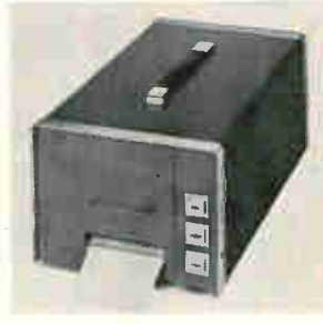
Digital printer series 2000 can print from 4 up to 20 columns at 60 lines per minute. Input may be from -30 to +30 v d-c with 100 kilohms input impedance and is BCD parallel entry 8421, 4221, or 2421. Designed for low-speed print-out systems, the rack-mounted model measures 7 x 19 x 15 in. Price is under $1,000. Digitron Corp., 2544 W. Main St., Norristown, Pa. 19401 [423]
