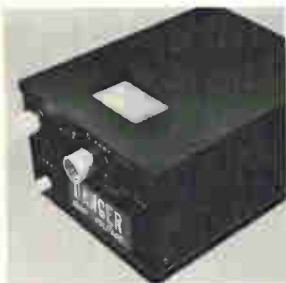
Sealed power supplies operate as a pair in character display crt systems. They operate from an input of 44 v d-c providing output voltages of 12 kv and -2.2 kv at \pm 1\% and 2 kv at \pm 5\% . Regulation is better than 0.25% for the 12 kv and -2.2 kv outputs and 1.5% for the 2 kv output with ripple on any output less than 0.1% peak to peak. AMP Inc., Elizabethtown, Pa. [385]
