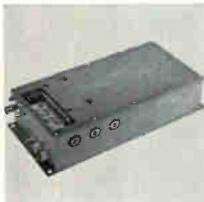
Crystal source FS-220 develops 1/2 watt at 3 Ghz with low a-m and f-m noise characteristics for communications use. It uses a 95-Mhz crystal oscillator as the base frequency followed by an amplifier/multiplier chain. Frequency stability is \pm 0.003% over 0° to +60°C. Unit meets MIL-E-5400 Class II for shock and vibration. Frequency Sources Inc., Box 159, N. Chelmsford, Mass. [405]
