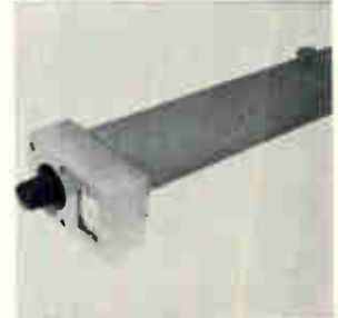
Four direct-reading, transmission type microwave octave wavemeters cover frequencies ranging from 970 Mhz to 12,430 Mhz. Insertion loss is 10 db max. Frequency readout is direct every 10 Mhz with accuracy of 0.1%. Spurious responses are 20 db minimum below desired response, and off resonance response is 40 db nominal. Gombos Microwave Inc., Webro Rd., Clifton, N.J. [404]
