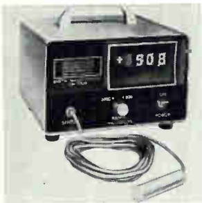
Digital flux-gate magnetometer model DM-2000 is for laboratory and industrial use. It displays ambient field values directly in milligauss on four non-blinking decimal readouts. A two-position switch selects ranges of either 200 milligauss, with \pm 0.1 milligauss resolution; or 2,000 milligauss, with \pm 1.0 milligauss resolution. Schonstedt Instrument Co., Reston, Va. 22070 [361]
