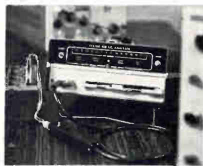
Troubleshooter. Instrument tests IC's without removing them from board.
