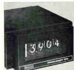
Digital frequency meter 4034 measures frequencies up to 1 Mhz and time intervals from 10 \mu sec to a million seconds. Heart of the unit is a crystal oscillator that establishes time intervals to an accuracy of \pm 0.01\% . The instrument's four-digit display allows it to count up to 9,999 cycles or time intervals. Beckman Instruments Inc., 2400 Harbor Blvd., Fullerton, Calif. [368]
