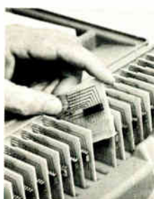
Select a reference board with a good IC that has the same type number.
