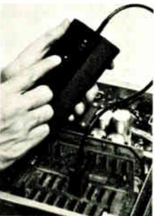
The suspect and reference ICs are compared automatically. Indicator lights signal which pins are faulty.
