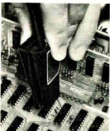
Attach the clip to the suspect IC and check the comparator display.
