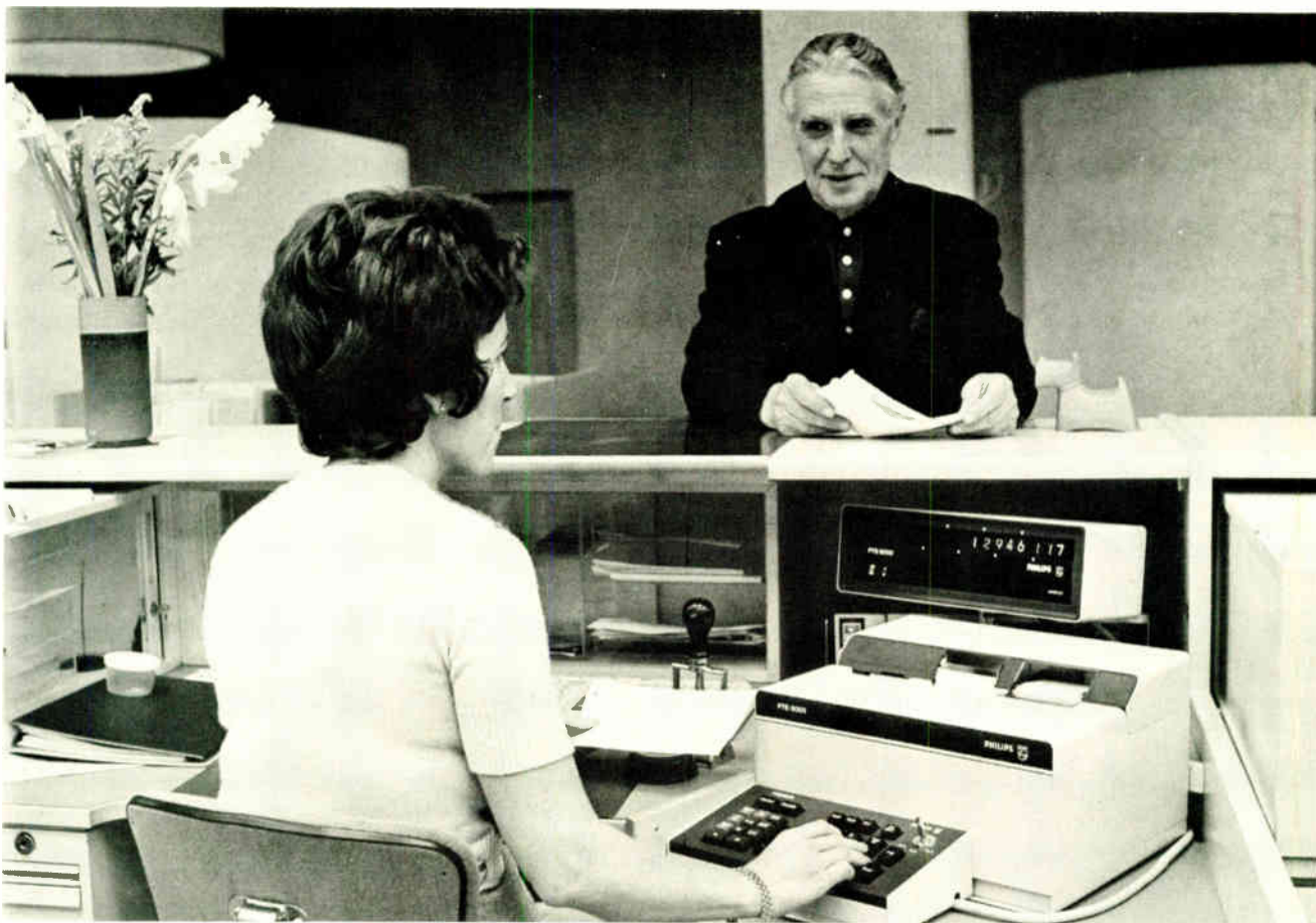
First of its kind. Cashier terminal in Svenska Handelsbanken's on-line teller system is initial installation in what will be a $12 million system. Transactions are registered and displayed and account information can be called from local, regional, and central files.
