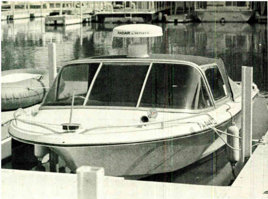
Resolution. Bonzer's radar for leisure craft offers high resolution over short ranges. The SR-20 has a peak output of just 40 watts, but that's enough for close-in detection.
