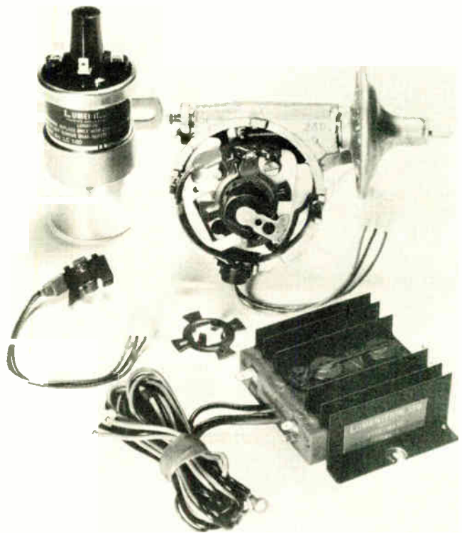
8. Low-cost ignition. Complete electronic breakerless-ignition conversion unit made by Autocar Electrical Co. Ltd. of England uses chopper inserted on distributor shaft and infrared emitter and photodiode. Breaking of beam by chopper is sensed by photodiode.
