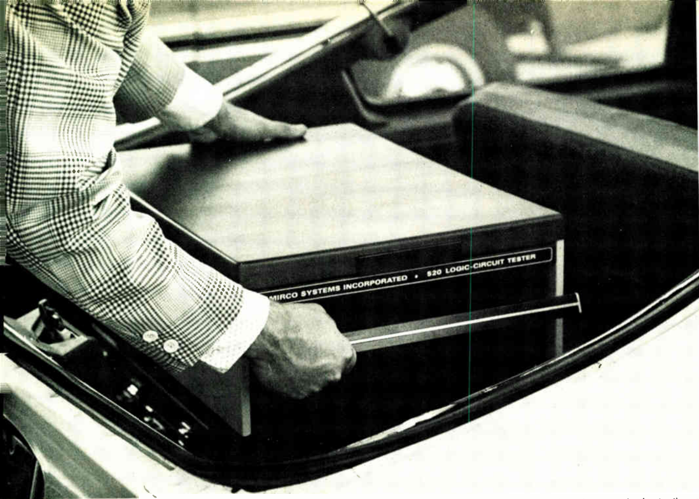
10. Tester for the road. Mirco's series 500 tester can provide field-service personnel with a potent portability advantage in the testing of logic circuits. The tester can be programmed at the user's discretion with both programed and pseudorandom test patterns.
