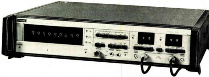
Debut. Femtosecond resolution of new time interval counter from United Systems Corp. should be useful for fusion lasers and in the design of high-speed logic families.
