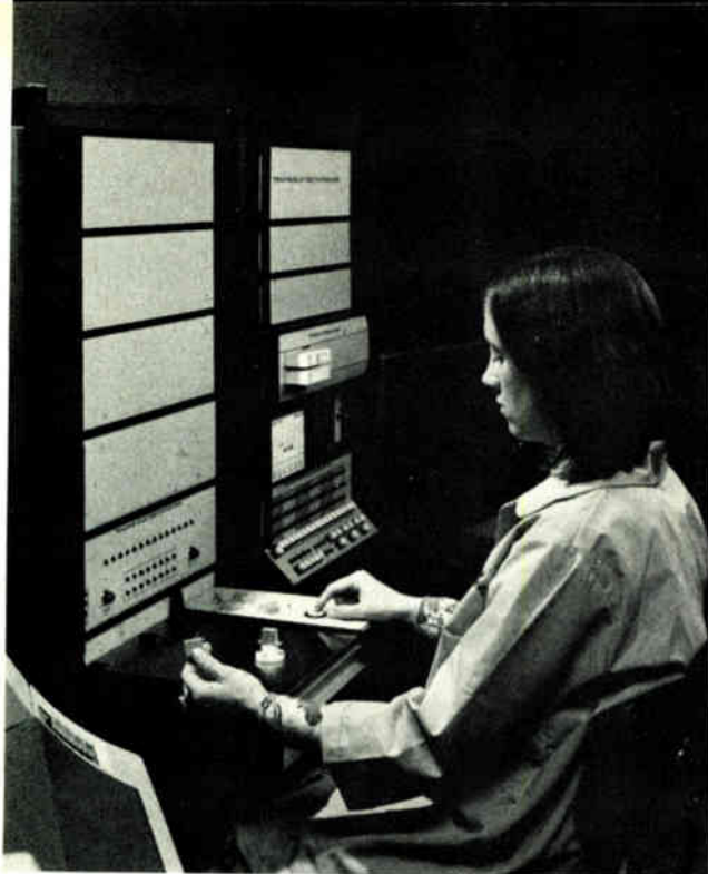
5. Component tester. Teradyne's K167B relay-test system is designed to examine a relay in any sequence with a single insertion. The system provides various types of hard-copy data that is valuable to the relay user and manufacturer.
