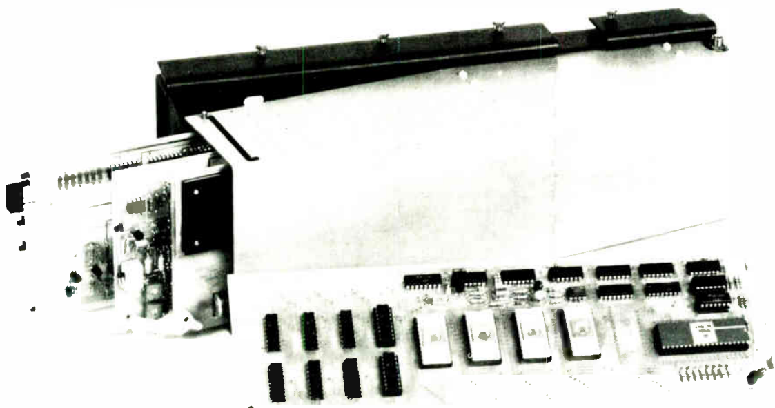
12. Flexible dialer. The four printed-circuit cards of the speed-tone dialer can be programmed to provide other functions as well. The controller card in front houses a 6800 microprocessor, four PROMs, and two C-MOS RAMs with additional sockets on board for six more.
