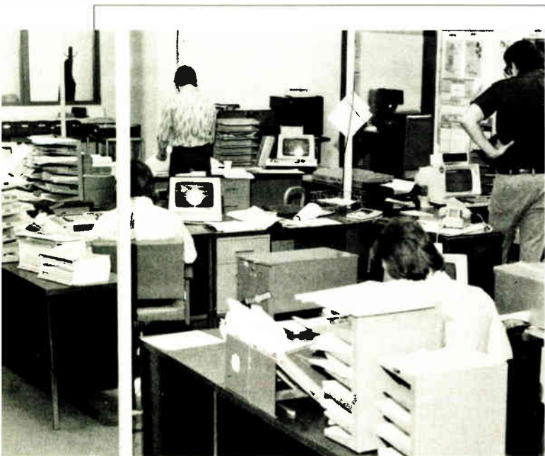
Computerized information systems, such as this one at Sterling Electronics, link the sales desk with regional warehouses, so the salesman knows instantly what is in stock, how much it costs, where it is and when more will arrive, so he can get components en route on the same day the order is placed.
