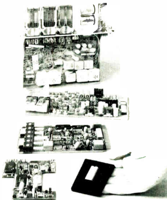
13. User's choice. The custom LSI digital timing chip in the hand forms the heart of two Collins Radio single-frequency signaling units: the "piggy-back" version (lower left) that plugs directly into a Collins channel multiplex modem, and the stand-alone version directly behind. Above the stand-alone version is its Collins predecessor that updated the Western Electric signaling module (top).
