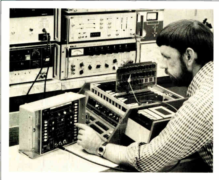
Digital troubleshooting. The Data Test Corp. tester combines a digital multimeter with a digital counter-timer in one package for troubleshooting digital systems.
