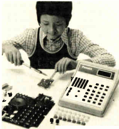
Easy work. Microcomputer kit is designed for fast assembly by school-age builders.
