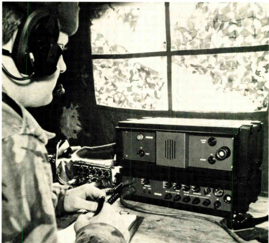
Flick of a switch. Frequency selection in Racal field transceiver is programmable for quick channel selection. Any 10 frequencies in the range may be entered in a memory.
