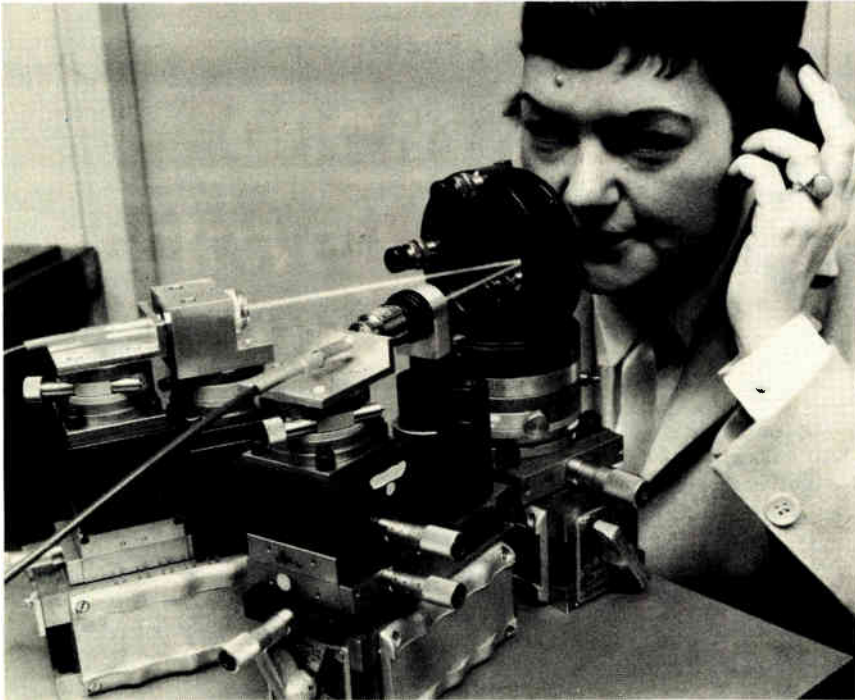
Light listener. Siemens' Ingrid Fromm tries out laboratory setup of light-powered telephone. She is speaking into vibrating membrane developed to modulate light.
