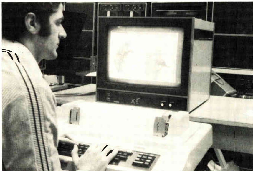
Colorful. Computerized angiography technique from DESY aids diagnosis of organ disorders by combining 128 X-ray pictures into one TV picture whose colors are a function of the rate of blood flow. Color scale at top (barely visible) eases interpretation.
