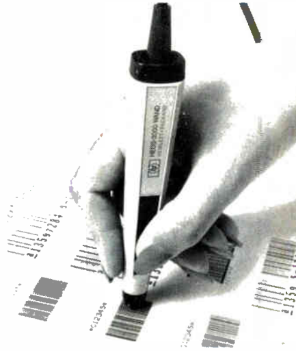
This new HEDS-3000 Digital Bar Code Wand is designed to scan black-and-white bar code and output TTL and CMOS-compatible signals. The heart of the wand is an advanced, high-resolution, high-speed, emitter/detector sensor in a sealed module near the removable tip.
