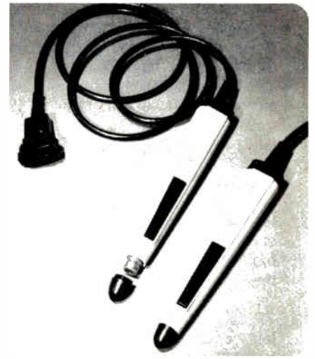
This new HEDS-3000 Digital Bar Code Wand is designed to scan black-and-white bar code and output TTL and CMOS-compatible signals. The heart of the wand is an advanced, high-resolution, high-speed, emitter/detector sensor in a sealed module near the removable tip.
