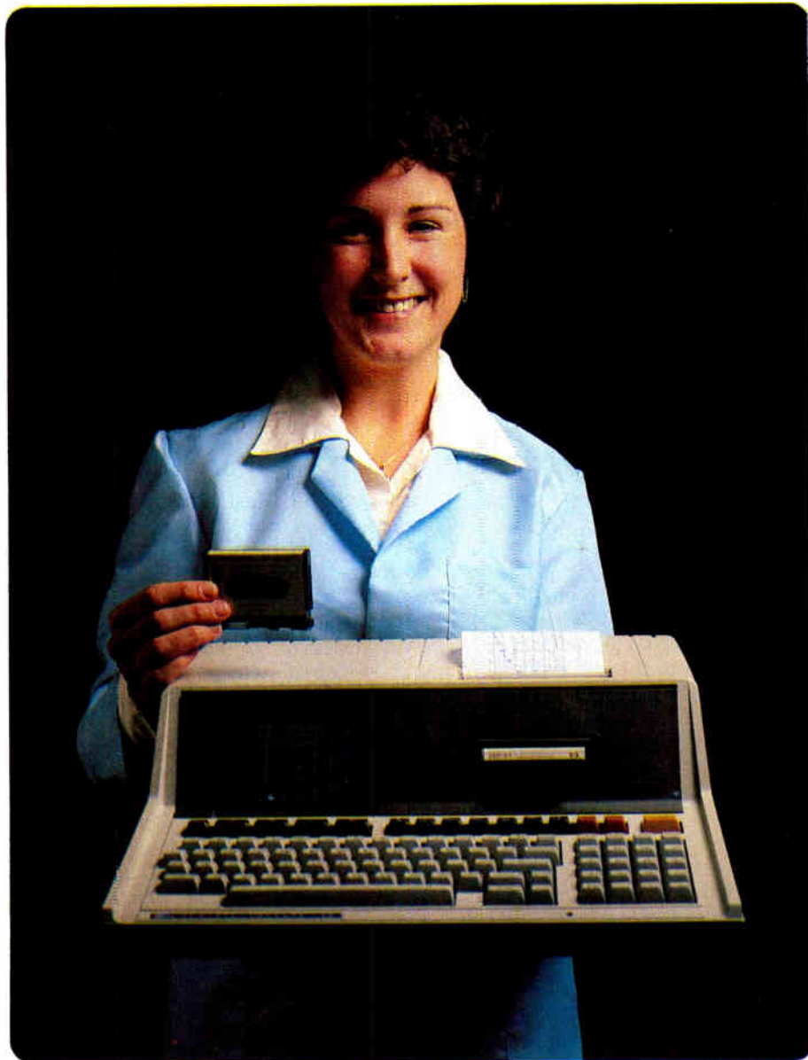
The HP-85 computer weighs a mere 20 pounds (9 kilograms). It's a very BASIC computer designed for individual use, with interactive graphics, expandable memory, optional peripherals, and interfacing potential disproportionate to its modest price.
