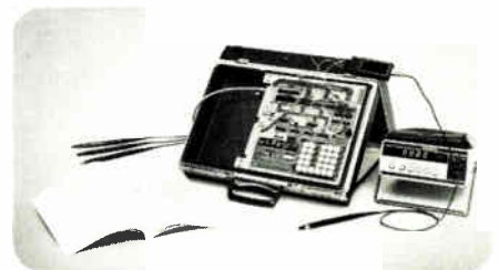
The 5036A Microprocessor Lab with optional 5004 Signature Analyzer and 5024A IC Troubleshooters Kit provide actual hands-on microprocessor troubleshooting experience.
