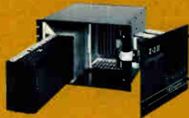
Hard disk drive at lower left can be interchanged just by sliding out and disconnecting plug. Seven free card slots are available. Z-2H includes printer interface card.
