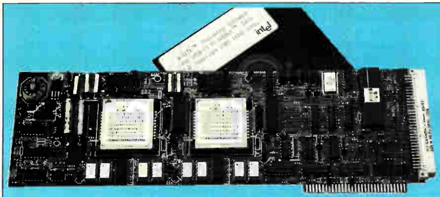
PERSONAL BUBBLES. The Intel PCB-75 bubble-memory board for the IBM Personal Computer and compatibles allows many users to easily evaluate bubble-storage technology.
