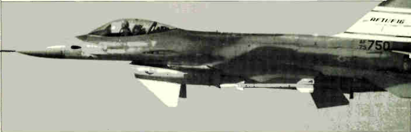
POD ON THE PLANE. Westinghouse's laser sensor/tracker pod mounts where the wing meets the fuselage on the F-16 test plane.
