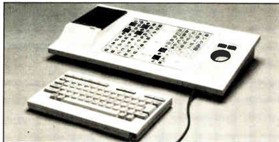
AI FOR THE MASSES. Sega's AI Computer will run computer-aided-instruction software written in Prolog.
