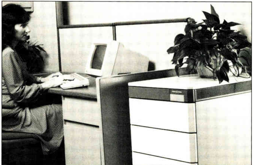
FILING CABINET. General Electric's Gefile system uses special-purpose VLSI processors to search through a text data base at much higher speeds than software-based systems can.
