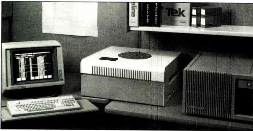
ASICs TOO. One version of Tektronix' DAS 9200 helps design and test ASICs.
