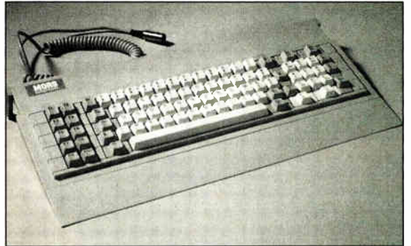
EASY TOUCH. A polyester film layer makes Mors's capacitive keyboard less expensive than pc-board-based competition.
