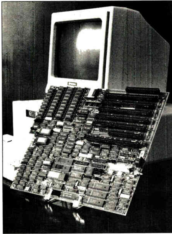
DOUBLE UP. The ET 286 Plus CPU board can carry a daughterboard with an 80287 coprocessor and fast peripherals.
