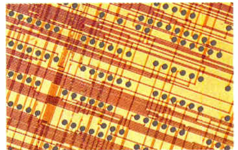
Advanced processing technology provides superior buried microvias in multilayer printed wiring boards.
