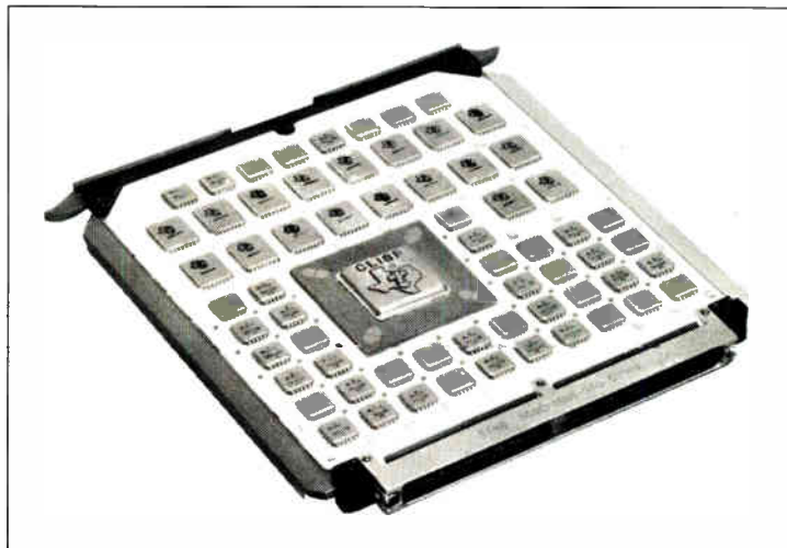
1. COMPACT LISP. The processor module is one of the five basic 6.58-by-5.88-in. military-style modules in Aries.
