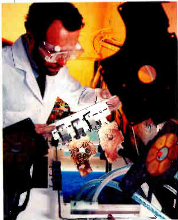
A GE technician prepares to dip a molded 3-d pc board into a fixing bath.
