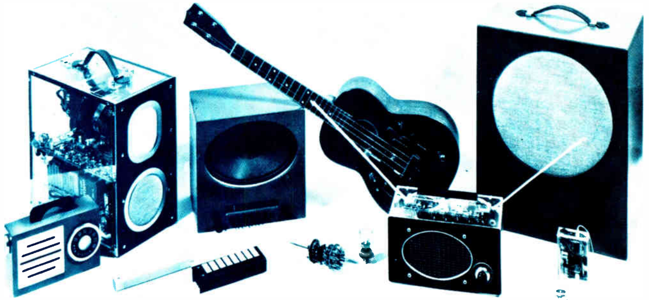
Transistorized. To prove the viability of transistors, RCA built prototypes of all-transistor radios, a TV set with a 5-inch screen, even an amplifier for an electric ukelele. The equipment was years from commercial production, though, since transistors then cost $15 or more.
