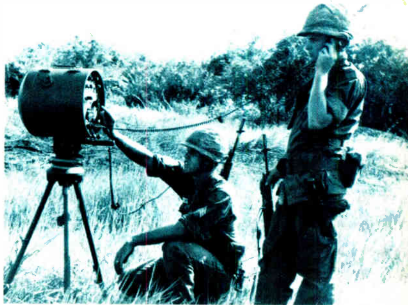
Silent Sentry. That was the nickname of the AN/PPS-4 portable combat surveillance radar produced by Sperry Gyroscope Co. in the mid-1950s. With a usable range of up to 5,000 meters, it converted radar returns into audible signals using a pulsed doppler principle.
