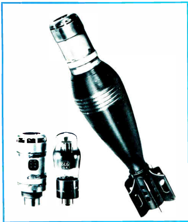
Microminiaturization's debut. The proximity fuze, shown here mounted on an 81-mm mortar shell, required radically new techniques for producing ruggedized miniature circuitry, such as screening and firing components on ceramic substrates.
