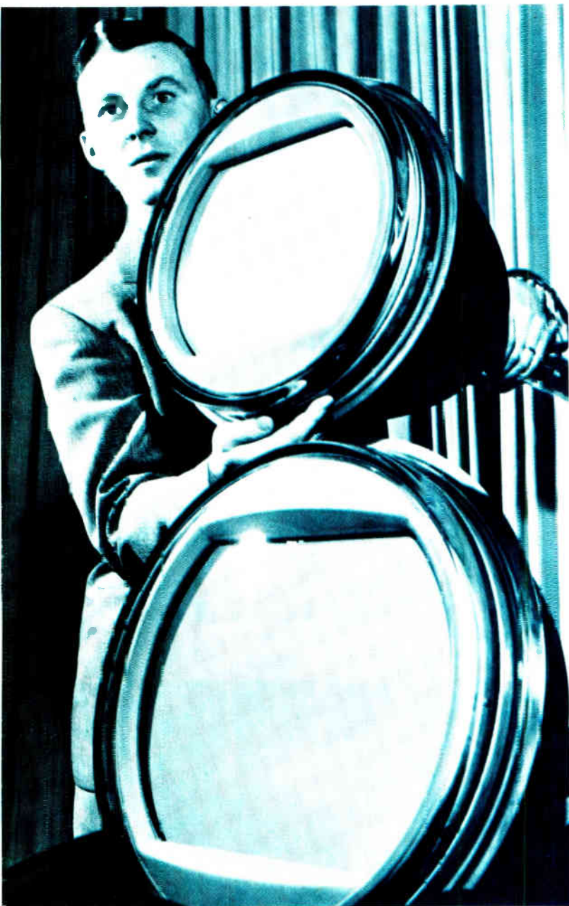
In color. Color TV began to move once the FCC adopted in 1953 the National Television Standards Committee's recommendation of the dot-sequential system. RCA's shadow-mask color tube helped black-and-white compatibility. This is a 19-inch 1954 version.
