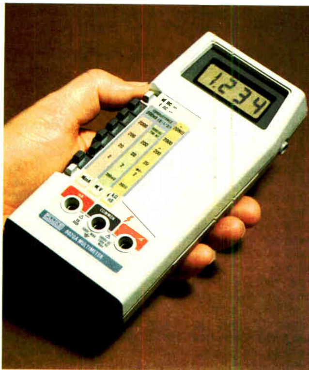
Attractive. Low-power liquid-crystal displays found their way into devices other than watches. Here they are being applied to one of the first hand-held digital multimeters to be commercially successful, John Fluke Manufacturing's model 8020, introduced in 1977.
