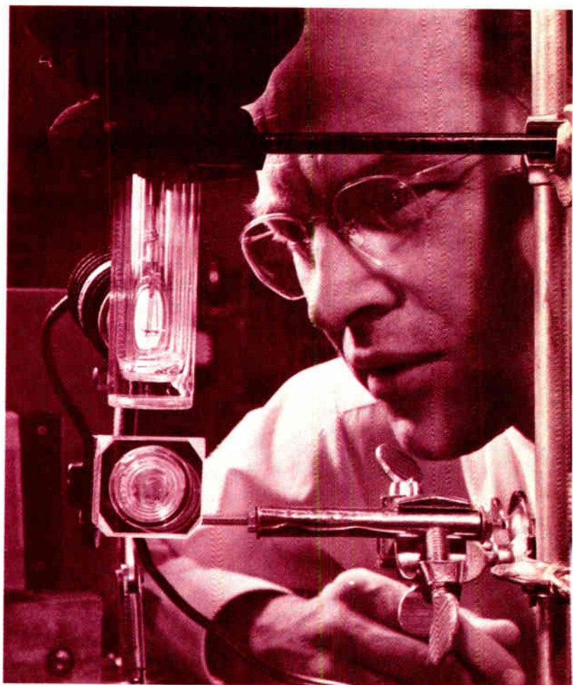
Laser. General Electric in 1962 had a new type of laser, one made of gallium arsenide, seen as a small spot between two electrodes within the circles at the lower end of the photograph. Robert N. Hall peers at his discovery, which was cooled in liquid nitrogen.
