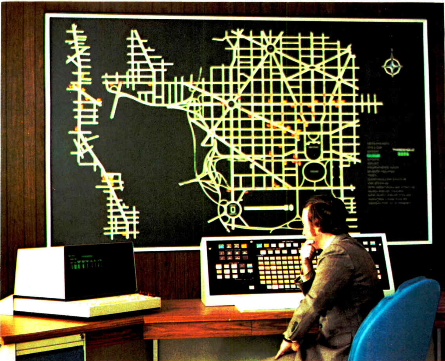
Controlling the wheels. At a traffic control center, which was used to determine the software needs of a computerized system designed by Sperry division of Sperry Corp., a controller tracks congestion on a major highway and at parallel intersections to divert traffic.
