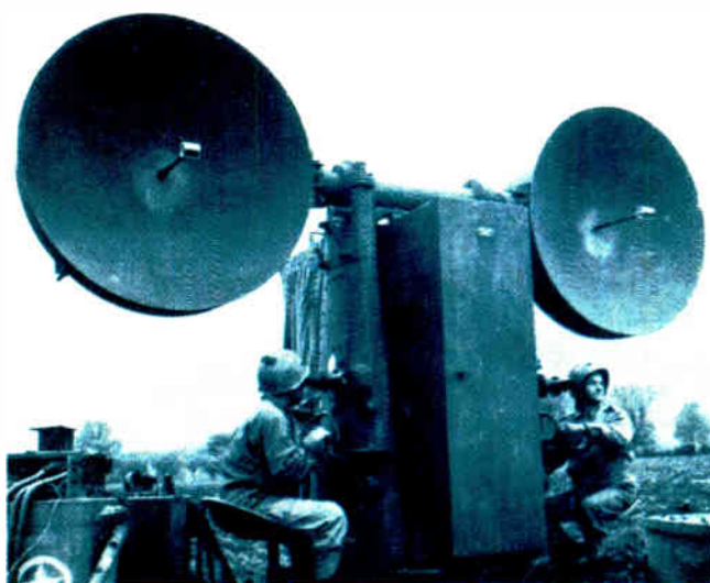
Mickey Mouse. Its twin antennas inspired the nickname of the U. S. Army's SCR-547 anti-aircraft radar shown at the front in Italy in 1945. It was designed to measure the height of enemy planes, the data being transmitted to a remotely located gun installation.
