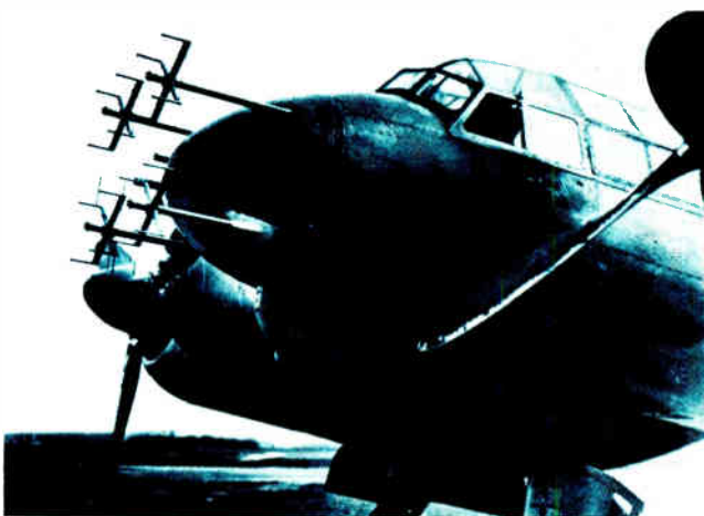
German radar. Antenna arrays built into the nose of this German plane are part of the airborne radar equipment used by the pilot to find his target during nighttime operations. Jamming from ground installations like Tuba proved an effective countermeasure.
