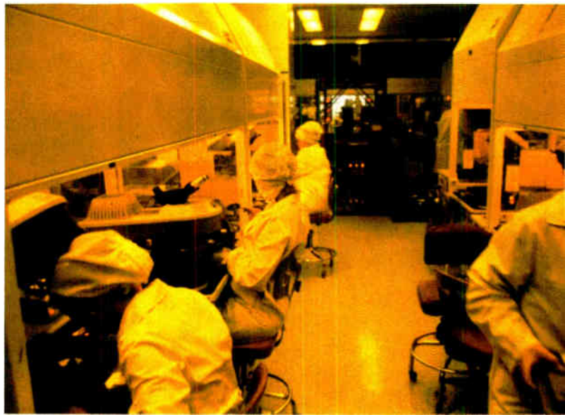
Glowing. The glow of yellow safety lights were features of the special lithography rooms, set up by every semiconductor maker, in which mask patterns were exposed on semiconductor wafers. Technicians in this American Microsystems facility are seen checking wafers.
