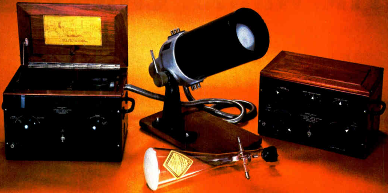
Scope. The cathode-ray oscillograph, as it was called, was introduced in 1931 by General Radio Co. (now GenRad Inc.). It came with power supply (left) and sweep circuit (right) that was also sold separately. The 2-foot-long tube, from Germany, had a screen 6 inches across.
