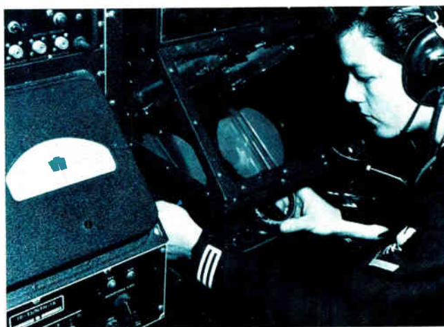
Touchdown. This is an early Navy version of radar air traffic control. The operator directs the plane from azimuthal position scanned on scope in front of him. Meter on left indicates deviation from center of runway. Another meter, not visible, records elevation.
