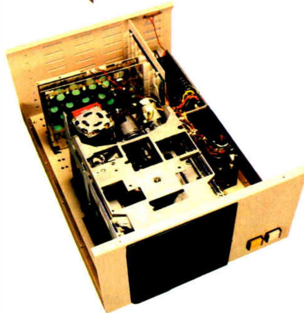
The C2-OEM with cover off showing the placement of floppy drives, UL recognized power supplies and 8-slot OSI 48 BUS backplane.
