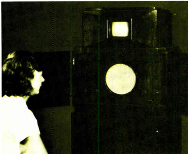
Big screen. Telefunken TV receiver, atop loudspeaker at 1932 Berlin Radio Show, was 9 by 12 cm, had 90 lines, 25 frames per second.
