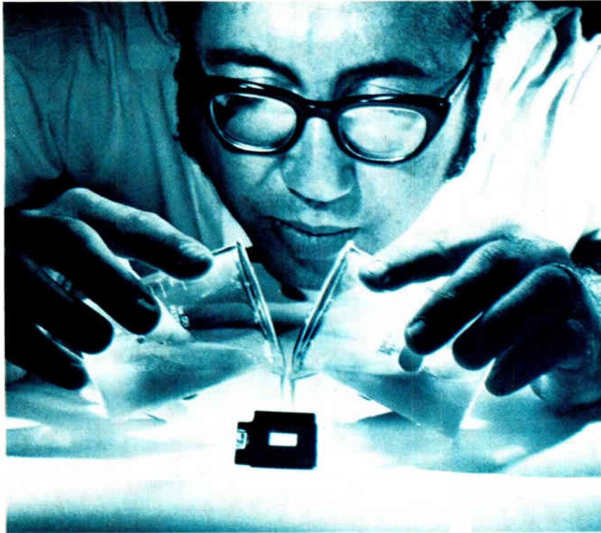
Alchemy. Liquid-crystal displays turned up in the sixties, promising low power and relatively large areas. RCA scientist Joel Goldmacher in this 1968 photo is pouring together two types of liquid crystal material to produce a quasi-emulsion that retains an image even after power is turned off.
