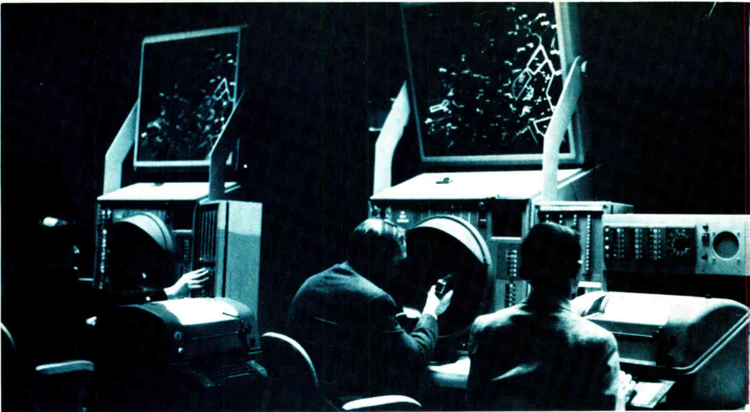
On guard. Computer-controlled operator consoles built by IBM were part of the high-performance ground radar system known as Sage, an ambitious aircraft defense system developed for the Defense Department, deployed in the U. S. and Canada, and linked by computers.
