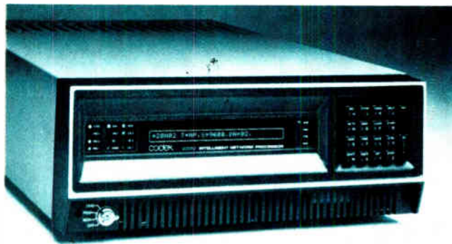
Decisions. Microprocessors gave digital communications nets many new capabilities. In 1975, Codex Corp.'s 6000-series Intelligent Network Processor examined data and made transmission decisions without customized programming and at radically lower cost.
