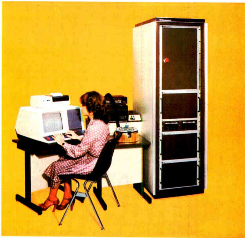
Tester. As new high-speed processes spawned memories with cycle times pushing 40 ns, ever faster testers were needed. Macrodata in 1979 first introduced a 25-MHz test system, the M-1, shown with its programming terminal, test fixture, and computer rack.
