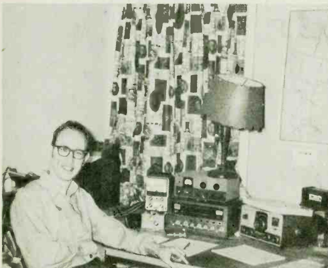
The black object at the right which looks like a can of paint, is really a dummy load. It is filled with oil, and during testing it dissipates the radio frequency output of the transmitter instead of allowing it to clutter the bands unnecessarily.
