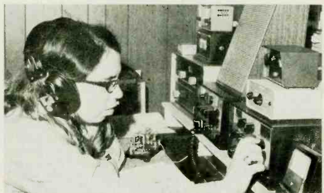
This high-quality station uses separate transmitter and receiver. The key used for code transmission in this setup is automatic, but works on a mechanical principle instead of an electronic one.
