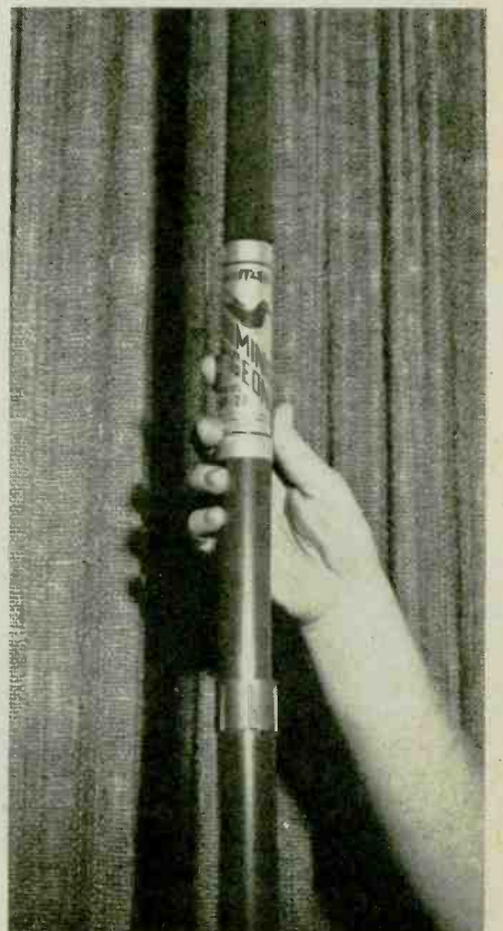
The antenna is tuned by decorative metal sleeves, adjusted for the best SWR reading.
