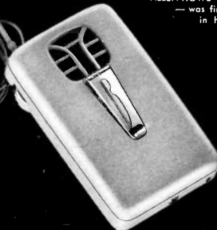
BELTONE — replaces 45 parts with one P. E. C. unit.
