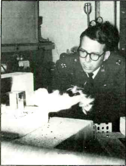
Fig. 6. An Air Force scientist looks on as a multi-kilowatt laser beam penetrates a plastic block. (Photo by Forrest Mims)
