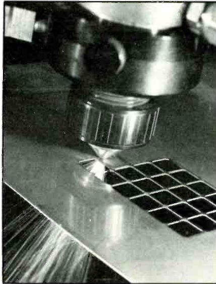
Fig. 7. A carbon-dioxide laser can weld, drill or (shown here) cut intricate patterns in a sheet of metal. (Courtesy Coherent Radiation)
