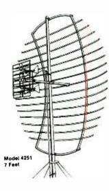
Channel Master's Model 4251 is a UHF-TV antenna using a parabolic reflector to direct signals to the 2 UHF antennas mounted in front. Reflectors behind the "bow ties" help increase gain. Overall length of this antenna is 7 feet. (Courtesy Channel Master)
