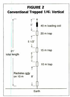
active element (see Fig.2)! By comparison, the HF-6V employs all of its 26 feet as an active element on 10 meters! (See Fig. 3 on next page.)The only band where a conventional trapped vertical will have comparable radiating performance with the HF-6V is on 40 meters, where both antennas use approximately 21 to 26 feet of vertical radiating element length.
