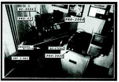
ment and the source of the noise. When I encountered interference, I lessened it by carefully lining the inside of my receivers with aluminum foil. Using double-stick adhesive tape to mount the foil, I was able to reduce most computer interference by about eighty percent.
