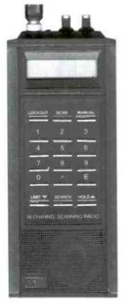
Figure 5. Electra Bearcat BC-100, the first programmable handheld scanner
