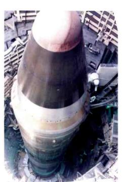
The Titan II stands 103 feet tall and is 10 feet in diameter. It is nearly 150 feet to the bottom of the silo.
