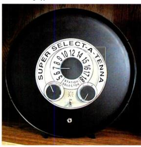
One of these applications involves coupling older model internal ferrite rod antennas that don't work well to this antenna to obtain good, high-Q, mutual coupling. My Sony 2010 tends to fit into this category and the Super-Select-A-Tenna did show a significant improvement over the second generation model I have been using with it.
