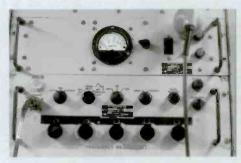
Close-up of the General Dynamics HF receiver-exciter and a wattmeter. Note the frequency reads out in "megacycles."
