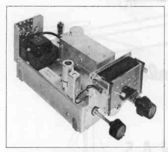
Figure 6. Chassis View of Dumont UHF Converter.
