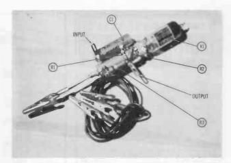
Figure 11. Cathode Follower Attachment on Vector Socket with Parts Indicated.
