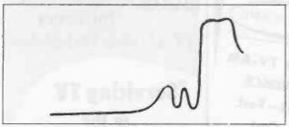
Figure 7. Improper Centering of Sweep Range. (Too low).
