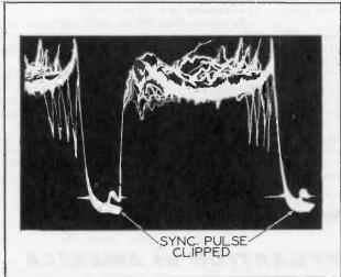
Figure 6. Video Signal Showing Results of Overloading. (Horizontal Sweep - 7875 cps.)
