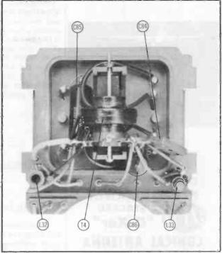
Figure 7. Horizontal Output Transformer
