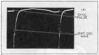
Figure 7A. Waveform at Output of Vertical Integrator Network - Picture "Locked-in."
