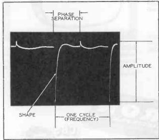
Figure 1. Waveform Showing Amplitude, Shape, Frequency, and Phase Separation of Pulses. (Horizontal Sweep - 30 cps.)
