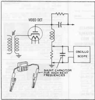
Figure 4. Capacitor for Sharpening Marker Pips.
