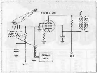
Figure 3. Dummy Antenna.
