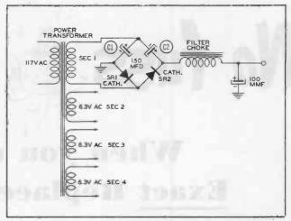
Figure 4. Full Wave Voltage Doubler Supply
