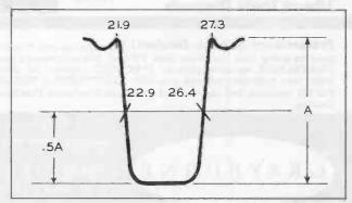
Figure 11. Overall Video IF Response for Motorola Chassis TS-172.
