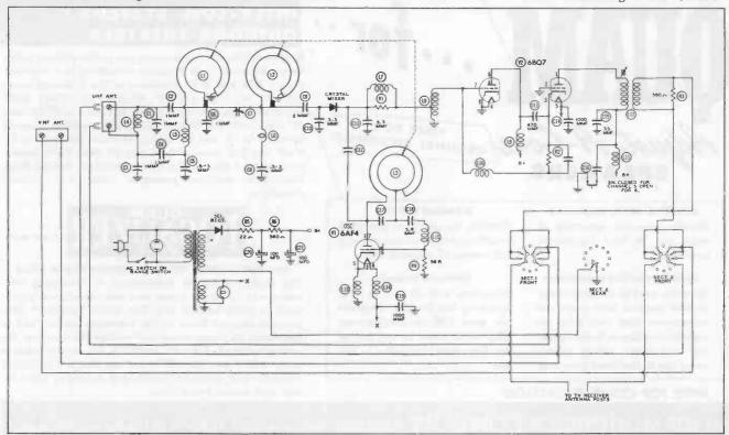
Figure 15. Schematic of Stromberg Carlson UHF Converter.
