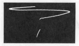
Figure 3. Lissajous Figure for Determining Frequency of Vertical Oscillator.
