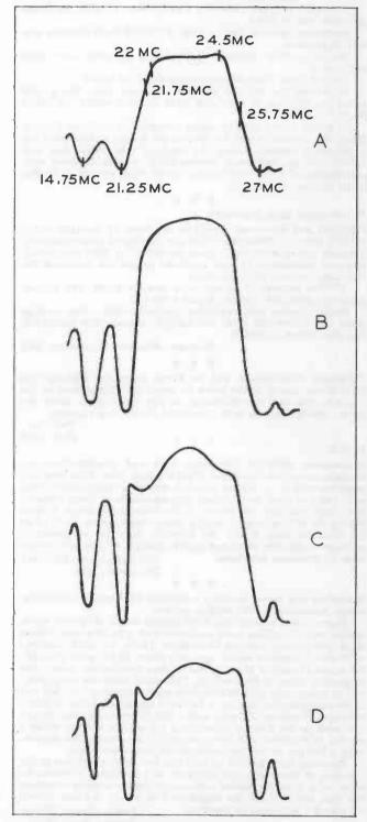
Figure 1. (A) Ideal Response Curve. (B) Bias at -2.5 Volts. (C) Bias at -2.0 Volts. (D) Bias at -1.5 Volts.
