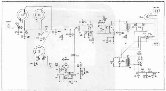
Figure 4. Schematic of Crosley UHF Converter.
