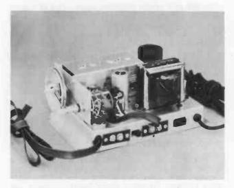
Figure 14. Chassis View of Stromberg UHF Converter.
