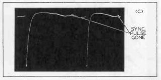
Figure 7C. Waveform at Output of Vertical Integrator Network - Picture not "Locked-in" Due to Loss of Sync Pulse.
