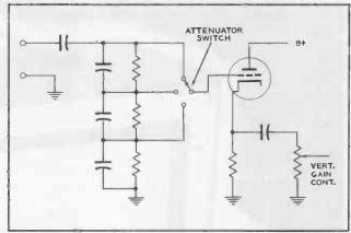
Figure 7. Typical Vertical Input to Oscilloscope Employing Cathode Follower Stage.
