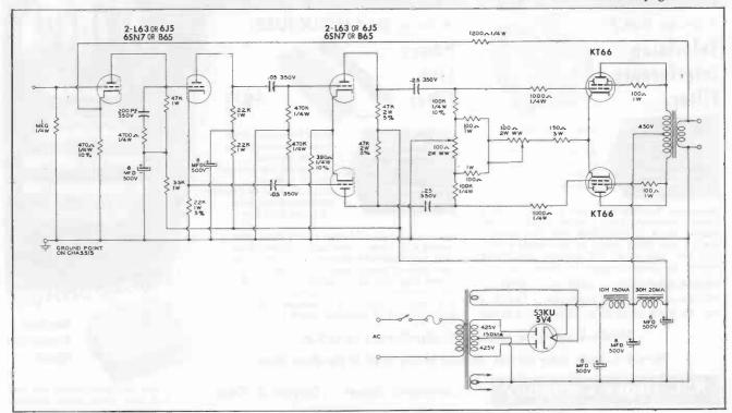
Figure 2. Schematic Diagram of Basic Williamson Amplifier.
