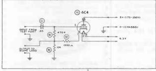
Figure 10. Schematic of Cathode Follower Attachment.
