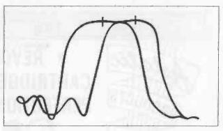
Figure 4. Sweep Generator Phasing Control not Properly Adjusted.
