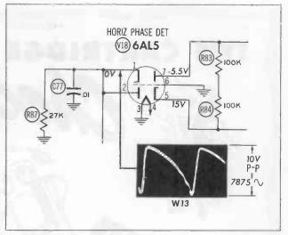
Figure 4. Sample Waveform from Photofact Folder. whole operation can be revealed through waveform investigation with an oscilloscope.
