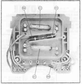
Figure 6. High Voltage Rectifier Tubes
