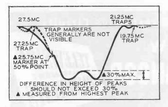
Figure 12. Overall Video IF Response for Admiral 24 D, E, F, G, and H Series TV Receivers.
