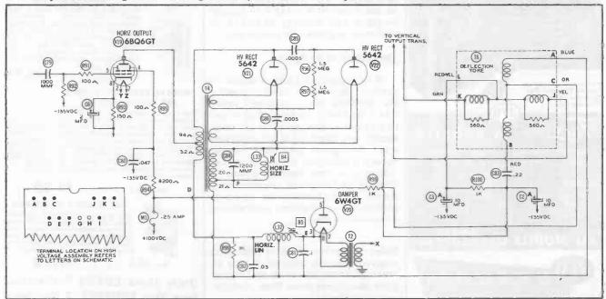
Figure 8. Schematic Diagram of Sylvania Ch. 1-260 Horizontal Deflection Circuit.
