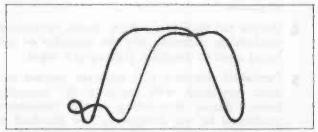
Figure 5. Insufficient Sweep Width for Phasing.
