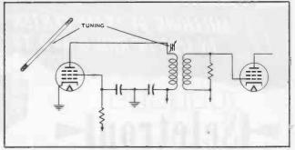
Figure 5. Tuning Wand for Touch-up Adjustments.
