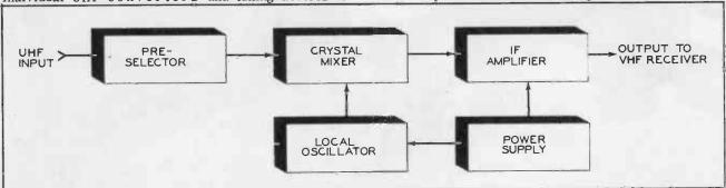
Figure 1. Block Diagram of a Typical UHF Converter.
