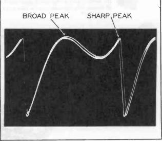
Figure 2. Waveform in Synchroguide Circuit Showing Broad and Sharp Peaks of Equal Height. (Horizontal Sweep - 7875 cps.)
