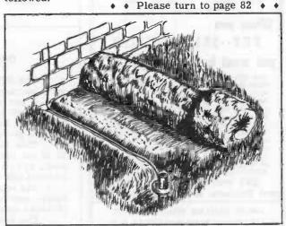
Figure 14. Procedure for Use when Driving Ground Rod in Lawn Several Feet From House.
