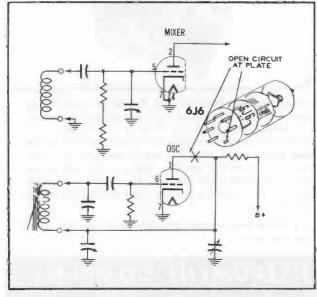
Figure 1. Dummy Converter.
