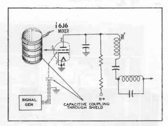
Figure 2. Ungrounded Shield for Dummy Converter.
