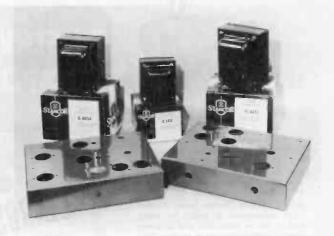
Figure 4. Stancor Components Used in the Williamson Circuit.
