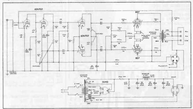
Figure 5. Schematic Diagram of the Stancor-Williamson Amplifier.
