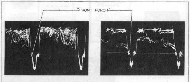
Figure 5. Composite Video Signal at Video Detector Load. (Horizontal Sweep - 7875 cps.) (A) On Narrow-Band Scope. (B) On Wide-Band Scope.
