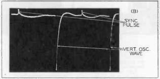
Figure 7B. Waveform at Output of Vertical Integrator Network - Picture not "Locked-in."
