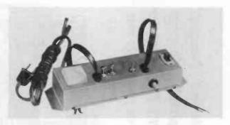
Figure 12. Sarkes Tarzian Single Channel UHF Tuner Unit with Self Contained Power Supply.
