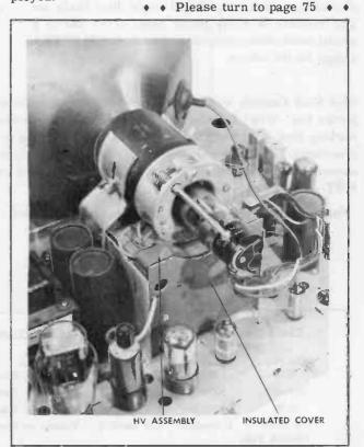
Figure 5. Packaged High Voltage Assembly
