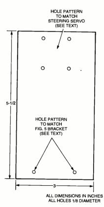
Fig. 4. The main body of "Elmer, Jr." is a simple piece of sheet metal.
