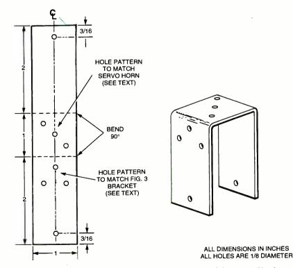
Fig. 1. The wheel frame is a U-shaped bracket formed from a piece of sheet metal. Use the servomotor and motor bracket as a guide when drilling their respective mounting holes.
