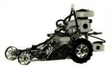
A combination robot/hot rod (another bonus plan available from the CyberK'NEX Web site). A motor is located at the rear of the robotic vehicle; a motor-control pad is located in the "driver's" seat.
