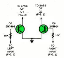
Fig. 4. If you add these transistors as indicated to the Fig. 3 circuit, you can prevent the bridge from burning out if you accidentally try to activate both directions at the same time.
