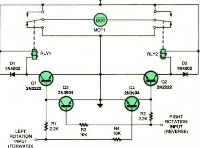
Fig. 2. If you want to control the relays of Fig. 1 with electrical signals, simply replace the switch with this transistor circuit. Note how one input automatically locks the other from activating.
