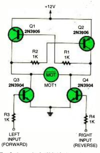
Fig. 3. A standard "H-bridge" configuration removes the mechanical contacts of a relay from the circuit, making for a more reliable circuit.
