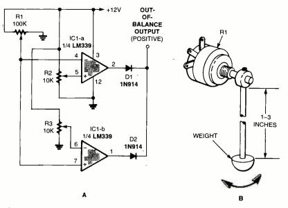
Fig. 8. Mounting a potentiometer with a pendulum-like weight gives your robot a sense of balance. If the unit is leaning too far in one direction, the circuit will output a warning signal. The clever robot builder will connect that output to a circuit that will help right the robot before it tips over.
