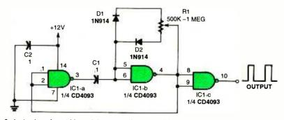
Fig. 5. A simple pulse-width modulator supplies a variable pulse width at a constant repetition rate—a good circuit for controlling the speed of a DC motor. The pulse width, set by R1, acts as the "throttle."
