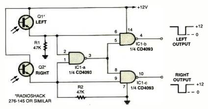
Fig. 7. A pair of phototransistors helps create a "steering" signal based on which transistor sees light.
