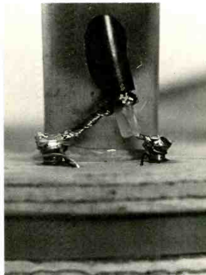
Fig. 10. Coax is routed to search coil through the shaft with ends soldered to the proper screws.
