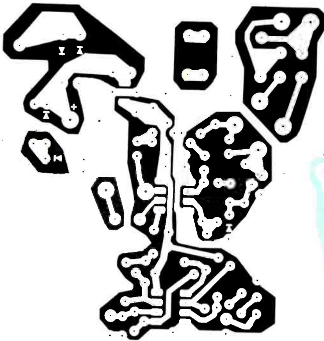
Fig. 4. Exact-size foil pattern (left) and component layout for the transmitter.
