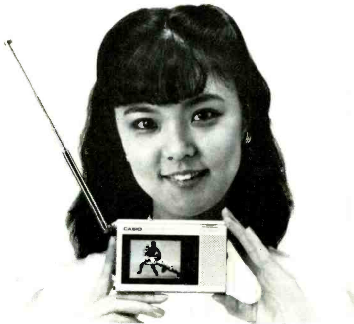
The Casio Model LCV-30 is 3\frac{3}{16} " \times 4\frac{11}{16} " and weighs 12.35 oz.
