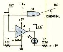
Fig. 4. If the mercury bulb in this circuit is tipped, UI-a will light LEDI by going low indicating a "tilted" condition.
