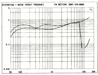
For mono reception, THD-plus-noise measured 0.4% at 1 kHz, while in stereo, THD-plus-noise was nearly 0.6% for the same modulating frequency.
