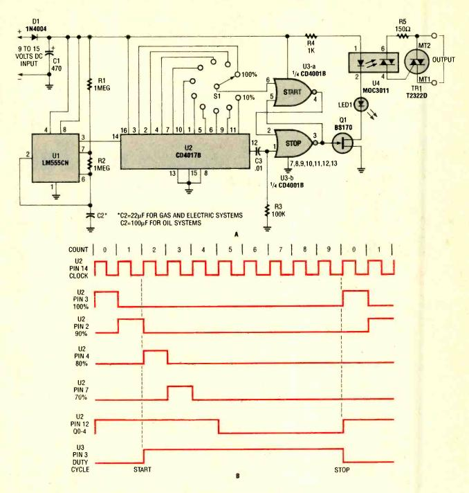
Fig. 1. Here are the schematic and timing diagrams for the Fuel Miser. The Fuel Miser is comprised of a 555 oscillator/timer (U1), a CD4017B decade counter/divider (U2), half of a CD4001 quad two-input NOR gate (U3), an MOC3011 optoisolator/coupler (U4), a BS170 N-channel, enhancement, TMOS field-effect transistor (Q1), a T2322D Triac, and a handful of support components.
