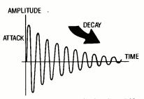
Fig. 6. With power applied, adjust R10 until the twin-T network is just about to oscillate; working from there, decrease R10's resistance until the circuit oscillates steadily. After that, increase R10's resistance until the oscillations fade to silence, as shown here.
