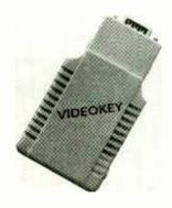
of the on-board VGA card, the Videokey allows any program to be viewed in a large, color format using readily available TV sets and broadcast-standard monitors. The device supports video modes of resolutions up to 640 × 480 with 256 colors. Interconnection is via RCA jacks or S-VHS connectors for improved resolution. All necessary cables and software drivers are included.
