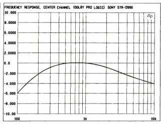
The response curve of the center-channel outputs when the surround sound "Normal" Dolby Pro Logic circuitry is used shows marked roll-off at both the bass and treble ends; that is deliberate and is called for by the Dolby Surround system to help emphasize spoken dialog.
