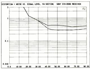
The THD-plus-noise versus signal-strength test was performed after a lengthy warmup of the receiver. Surprisingly, the stereo THD-plus-noise was actually lower (0.3%) than that of mono, which still measured 0.4%.
