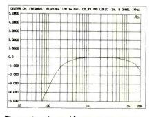
The center-channel frequency response in the Dolby Pro-Logic mode. This is typical of A/V receivers.
