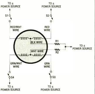
Fig. 1. This common 6-lead bifilar-wound stepper motor consists of two center-tapped windings. Note that the center tap of each winding is connected through a current-limiting resistor (RI or R2) to a power source.
