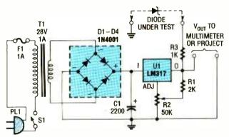
Fig. 1. This versatile circuit can be used to test Zener diodes or act as a stand-alone power supply. Note that it requires a voltmeter to work as a Zener tester.
