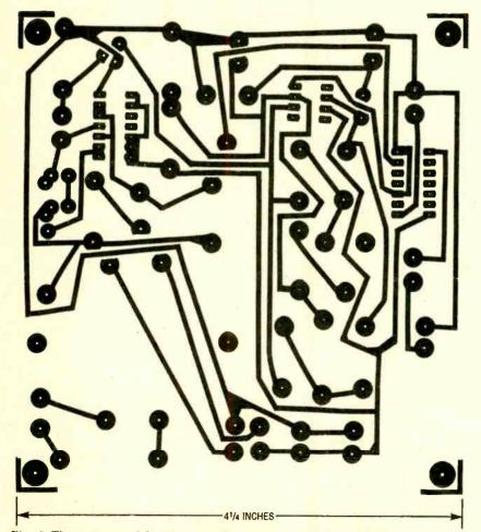
Fig. 4. The prototype of the Electronic Gong was assembled on a printed-circuit board, measuring approximately 4<sup>1</sup>/<sub>4</sub> by 4<sup>19</sup>/<sub>16</sub> inches. Here's a template of that foil pattern.
