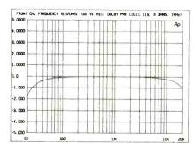
The frequency response of the front channel of the RX-V1050 A/V receiver in the Dolby Pro-Logic mode.
