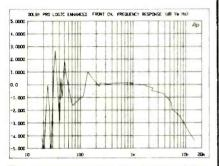
The enhanced-mode front-channel frequency response. Compare this to the standard pro-logic mode.
