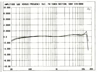
The frequency response of the FM tuner section was essentially flat (within  $\pm 1 \text{ dB}$ ) from 30 Hz to around 13 kHz, and exhibited an attenuation of around 4 dB for the left channel at 15 kHz and less than 2 dB for the right channel.
