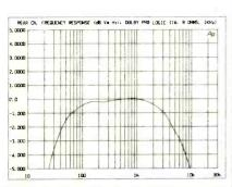
The rear-channel Pro-Logic frequency response. The Dolby specification calls for a roll-off at 7 kHz.
