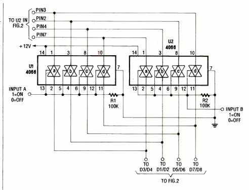
Fig. 5. The stepper motor's direction of rotation is reversed by reversing the drive delivered to the motor. That can easily be accomplished through this bilateral-switch control circuit.
