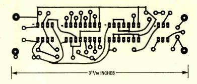
Fig. 2. The author's prototype was built on a small printed-circuit board, measuring about  $3^{11/6}$  by  $1^{3/4}$  inches; a full-size template of that printed-circuit pattern is shown here. You can etch your own board from the pattern shown or purchase one from the supplier listed in the Parts List.
