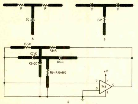
Fig. 3. The filter network is comprised of two separate T-filter elements—lowpass, A, and highpass, B, filters—which combine to produce a bandpass filter. The basic configuration for the twin-T filter used in the Electronic Gong is shown in C. Also shown is the relationship between the components values of the two filter elements.
