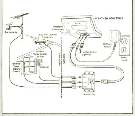
Fig. 1. Accurate weather readings depend upon proper installation of the Weather Monitor Il's sensors, wind vane, and optional rain-collector, as depicted in this illustration from Davis' excellent user's manual.
