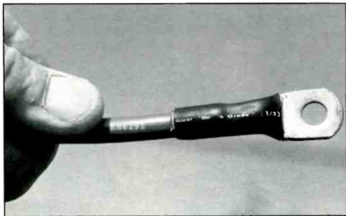
Reduce vehicle noise by bonding the hood to the chassis with braid or large cable.
