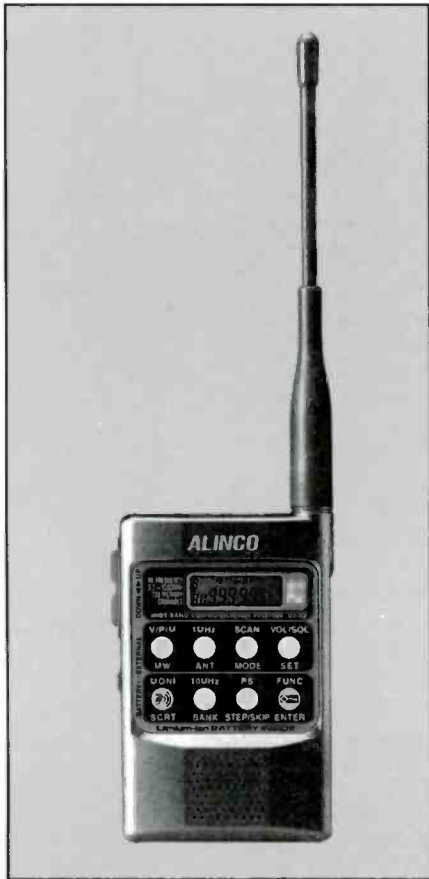
The Alinco DJ-X2 wide band multi-mode communications receiver.
