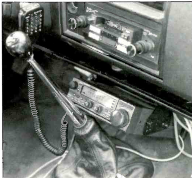
This radio was re-grounded for noise elimination. We noticed much less noise across the bands.
