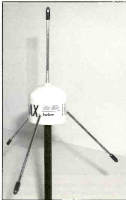
A 1/4 wave ground plane features a center vertical element, with "radials" around the bottom. Sometimes they're slanted downwards, and sometimes they are not. Three or four radials are common, but there are antenna designs with many more. Stick a magnet-mount antenna on a car's trunk lid or a filing cabinet to create your own ground plane.
