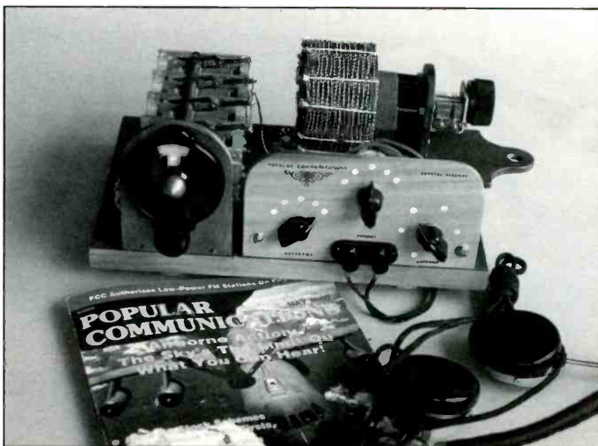
Reader John Haught's Lyonodyne crystal receiver. The white switch position markings are done by drilling holes to a 1/16" depth and then filling in the depressions with a white putty stick from the local hardware store.
