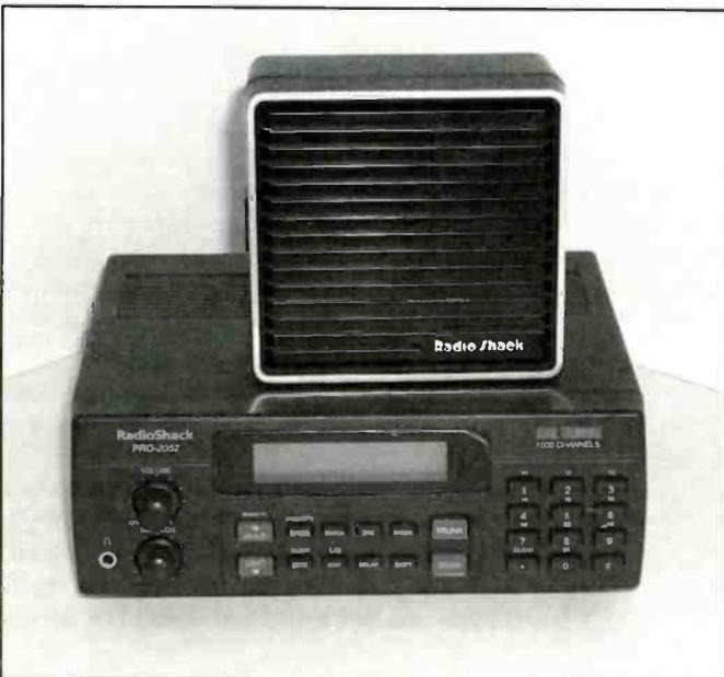
The larger speaker has a better sound, and this one is optimized for communications range. Don't hook it to your Walkman — you'll be very disappointed, but it will help your scanner considerably.
