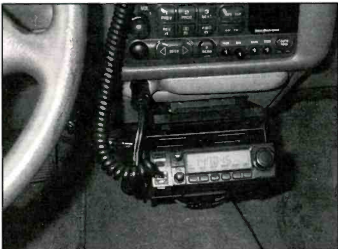
My ICOM IC-2100 mobile ham radio mounted to the Lumina's ashtray using the Gamber-Johnson Super Slide™ Slide Mount.
