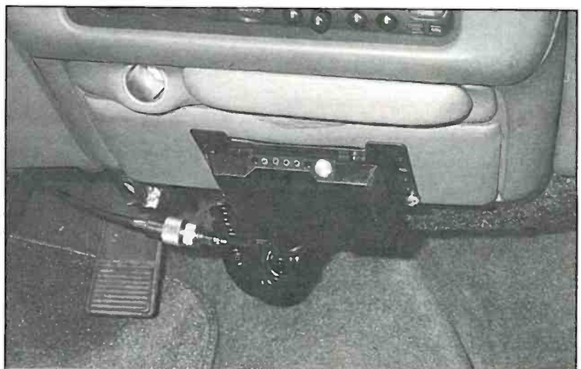
Here's a drawing taken directly from the box showing how the radio is mounted to the SS-100 slide mount.
