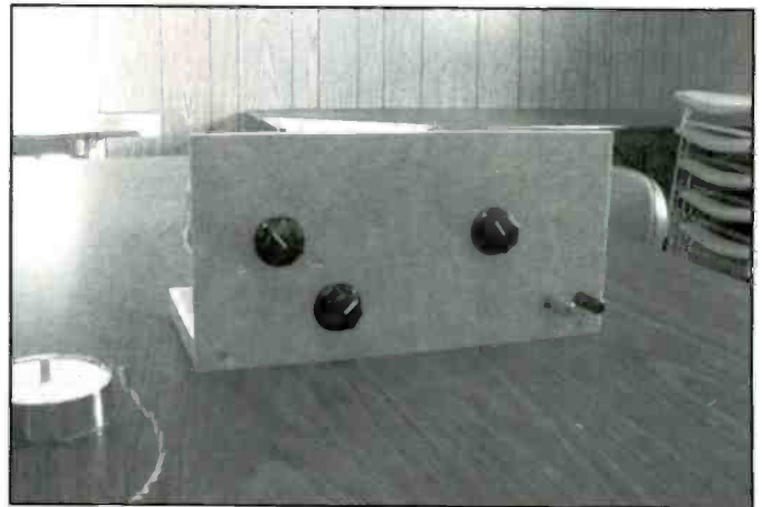
Earlier version of the Haynes receiver before the bandspread tuning was added.
