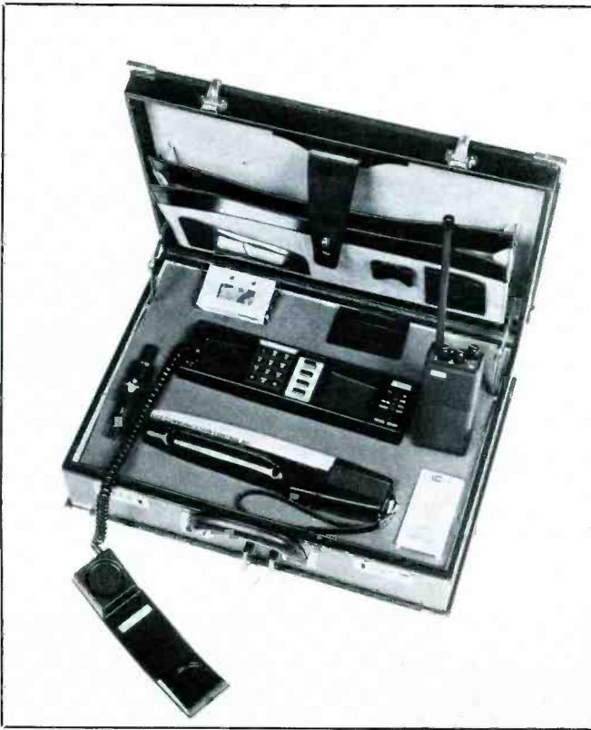
This portable secure-voice telephone system also contains detection components to let you know if the room is bugged or contains secret tape recorders. The case will sustain a direct hit from a .357 Magnum. (Courtesy CCS Communication Control, Inc.)
