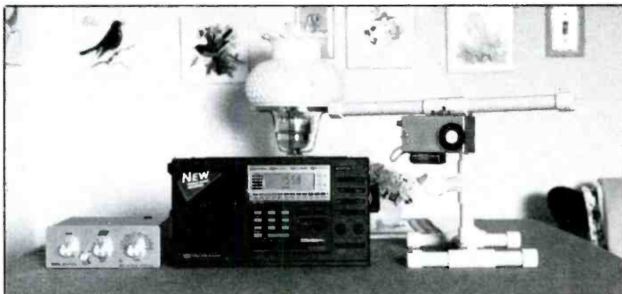
Fig. 4. Portable radio with tunable pre-amplifier and MW loop antenna. All can be battery powered
