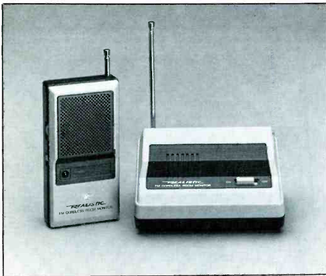
Wireless FM room monitors broadcast the sounds of a home as far as a mile or more. (Courtesy Radio Shack Division of Tandy Corp.)
