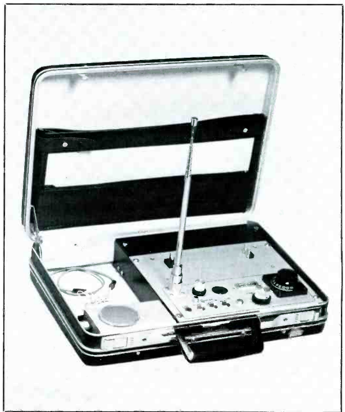
When you open this attache case, it reveals a sensitive transmitter detector that warns of any wireless room or telephone bugs, or nearby person wearing a hidden body transmitter (a "wire"). (Courtesy ESC.)
