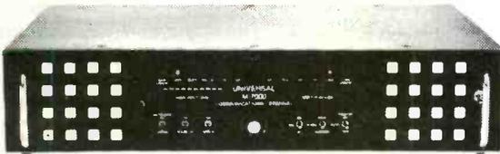
The Universal M-7000 will permit you to intercept and decode Morse code, various forms of RTTY, FDM and FAX. Simple connections to your receiver and video monitor will enable you to monitor with the most sophisticated surveillance decoder available. No computer is required. See the world of shortwave excitement you have been missing. Requires 115/230 AC 50/60 Hz. With video fax and real time clock only \$1159.00 *Please write for full details.*
