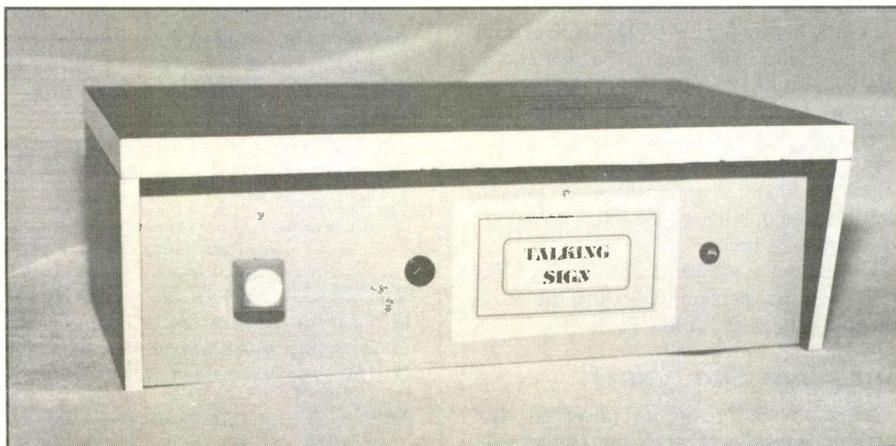
The FM-3 "Talking Sign" is a complete, self-contained, personal FM broadcasting station with a 200 ft. transmitting range. It doesn't require an FCC license. See text for further information.
