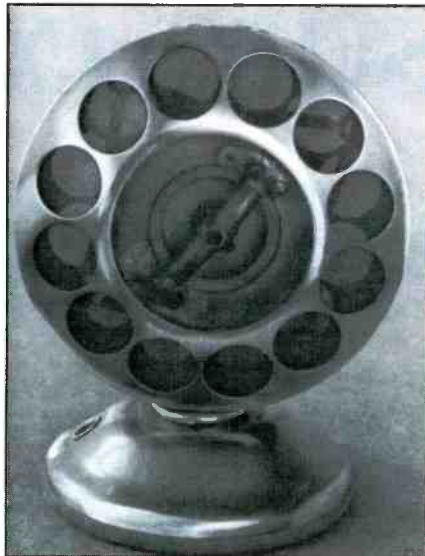
A double button carbon type microphone with two granule chambers and single diaphragm, as used until about 1927. A real museum piece.
