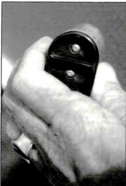
These two contact points will trigger the transmitter to "on" when moisture or melting snow make contact.
