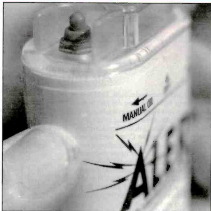
The ALERT 418-MHz receiver utilizes digital processing to minimize false sound-offs.
