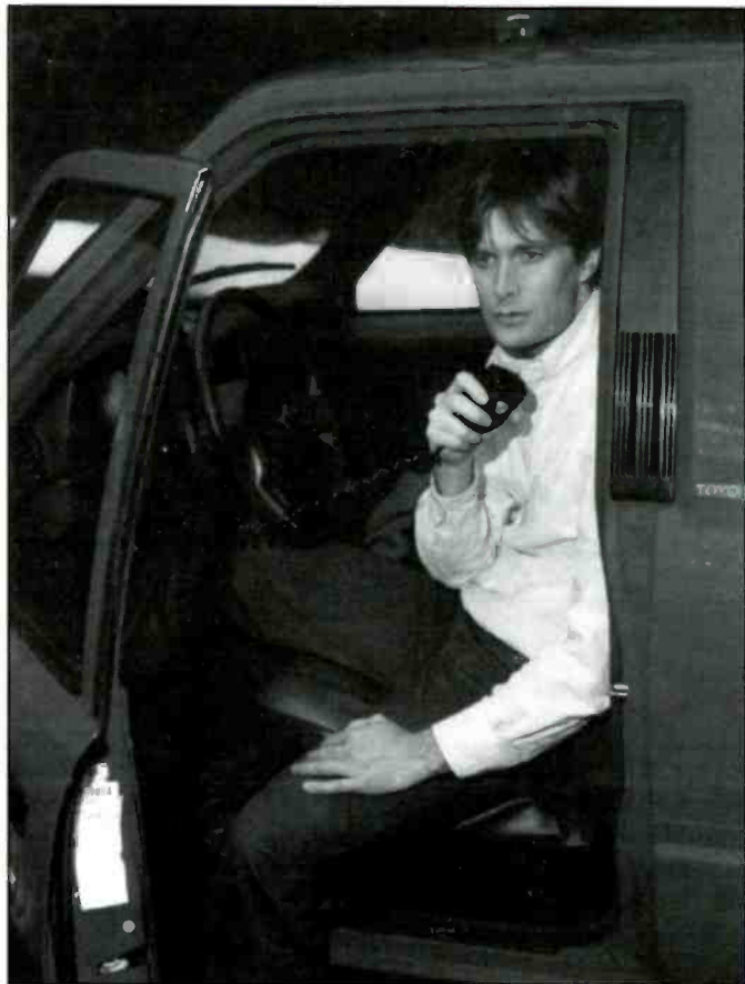
Hams often have the capability to place telephone calls over local VHF and UHF repeaters. Using a Touch-Tone pad on the radio or its microphone, both mobile and handheld amateur gear can become "mobile phones." (Photo courtesy of American Radio Relay League)
