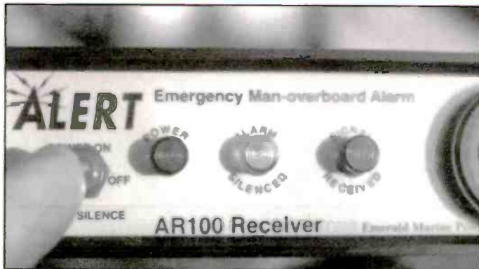
The ALERT 418-MHz receiver utilizes digital processing to minimize false sound-offs.
