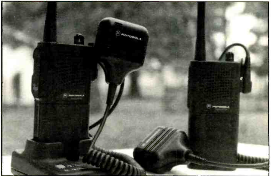
The Motorola Radius SP10 VHF transceiver is even more versatile with the accessory speaker-microphone. (Photo by Chuck Gysi, N2DUP)
