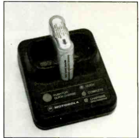
The optional quick charger base for the Radius SP10 can recharge the Motorola battery in three hours, or the standard 16 hours. (Photo by Chuck Gysi, N2DUP)
