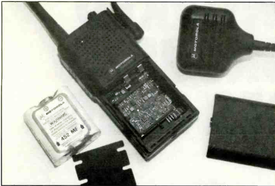
This is how you can reprogram the operating frequency of a Motorola Radius SP10 VHF handheld. With the battery compartment cover removed, lift out the rechargeable battery and the thin plastic cover underneath the battery. Notice the programming dipswitches inside the bottom righthand side of the radio. (Photo by Chuck Gysi, N2DUP)
